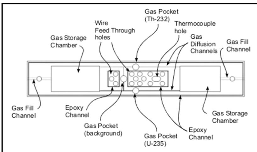
Figure 3. Aluminum oxide cavity (front view line drawing) piece showing the locations for feed-through wires, gas storage, diffusion channels, detector pockets, and the thermocouple. Additional epoxy channels were added to aid in bonding the parts together.
