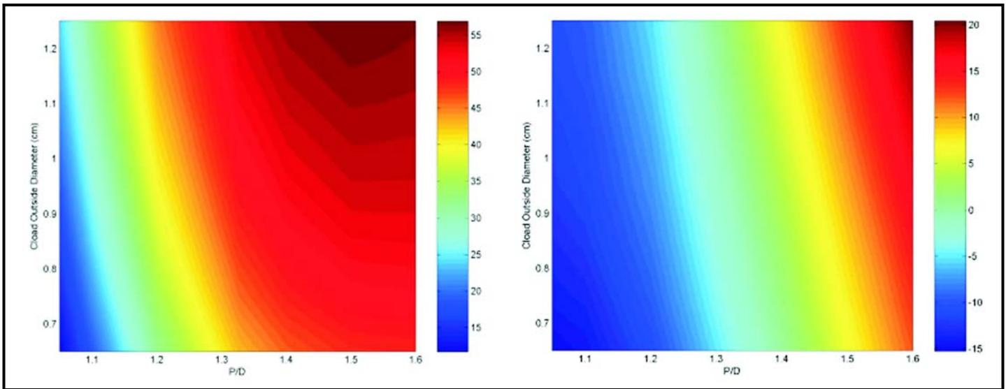
Figure 1. Attainable burnup (left) and coolant temperature coefficient of reactivity (right) for U-ThH<sub>2</sub>-ZrH<sub>1.6</sub> fuel having 55 volume percent ThH<sub>2</sub> and using 12.5 percent enriched uranium.
