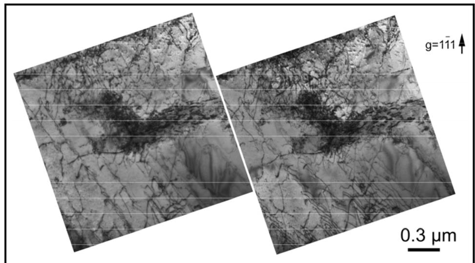
Figure 2. TEM brightfield stereo pair illustrating the crack-tip dislocation structure in an alloy 690 sample after exposure to Pb-doped caustic environment.
