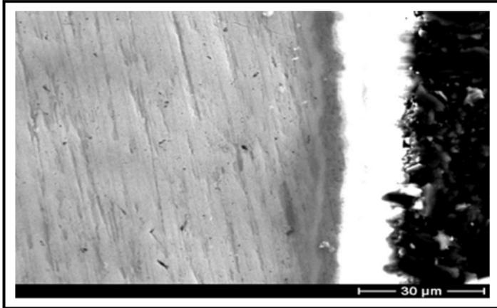
Figure 1. Growth of the oxide corrosion product layer of  $N^+$  ion implanted Zircaloy-2 after exposure to supercritical water at 500°C for 7 days. An oxygen diffusion zone is observed in the underlying alloy. Erosion of the oxide due to the flow of supercritical water was also observed.
