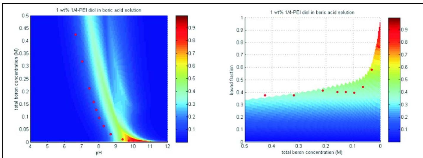
Figure 1. Results using Simple Ion Pairing Model: This model describes most of the behavior of the system. Researchers calculated the surface. The red dots represent experimental data. The color axis represents the fraction of total boron bound by the polymer.
