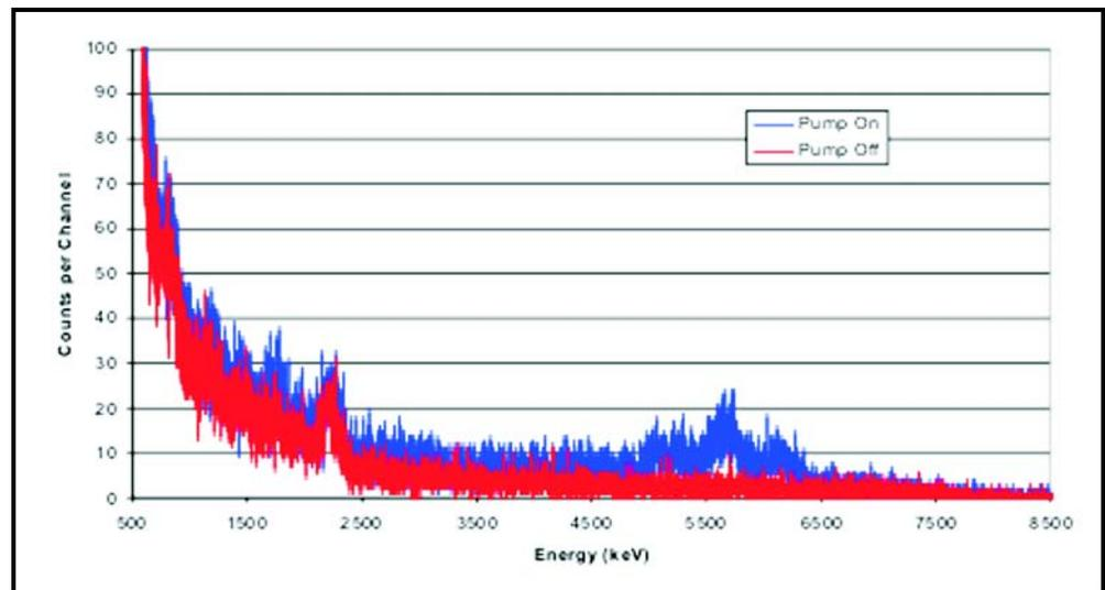
Figure 2. Experimental <sup>16</sup>N gamma-ray spectra detected by a Bismuth Germanate detector when circulation pump is on or off. The 6128.6-keV <sup>16</sup>N gamma ray plus the single- and double-escape peaks are clearly visible in the pump-on case.
