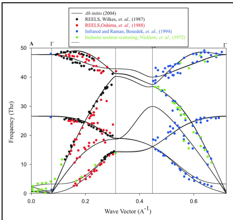
Figure 1. The dispersion relations for graphite as compared to experimental data. The calculation is based on a  $6 \times 6 \times 1$  supercell model and a  $3 \times 3 \times 4$  k mesh.
