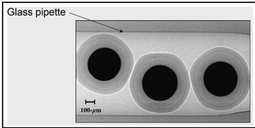
Figure 2. Cropped radiographic image obtained in analyzing and preserving the identity of about 20 particles stacked end-to-end in a thin-walled glass pipette.
