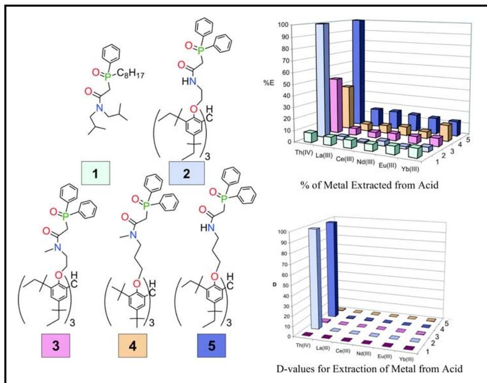
Figure 1. Extraction properties of the CMPO ligands developed at University of Florida.
