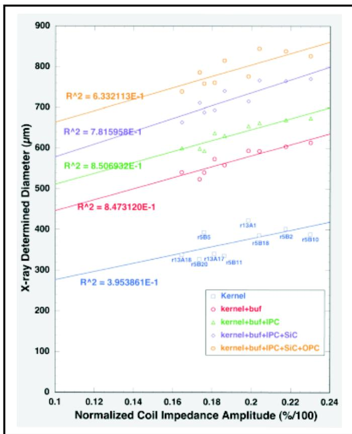
Figure 4. Radiographically determined coating layer diameter and induction coil impedance measurements.
