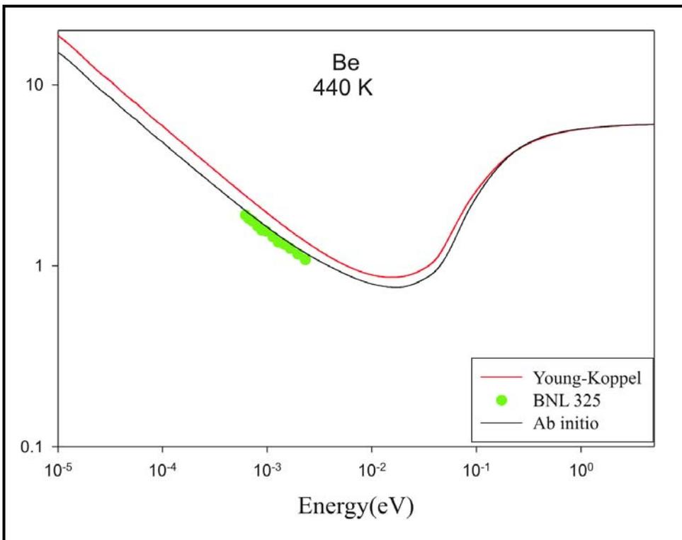
Figure 4. The impact of the one-phonon coherent inelastic scattering component on the inelastic scattering cross section of Be.
