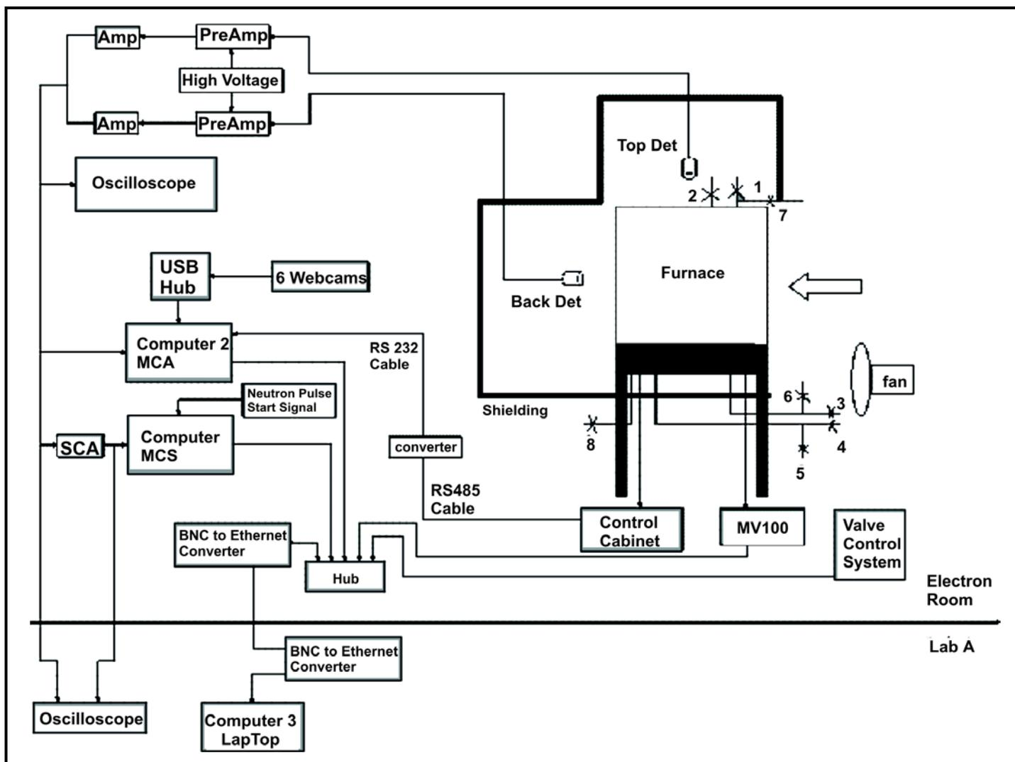
Figure 5. A schematic of the graphite experiment as it currently stands at ORELA.
