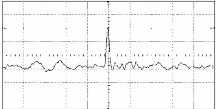
Figure 1. The preamplifier output with a voltage scale of 50 mV/div and a time scale of 5 ns/div.
