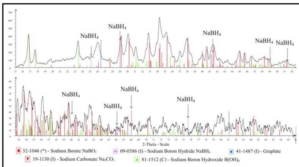
Figure 5. X-ray diffraction trace for the reaction product.
