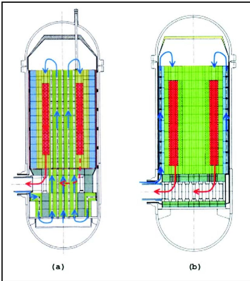
Figure 1. GT-MHR reactor vessel configured with alternative inlet flow paths. (a) Flow routed through central reflector. (b) Flow routed through permanent side reflector.
