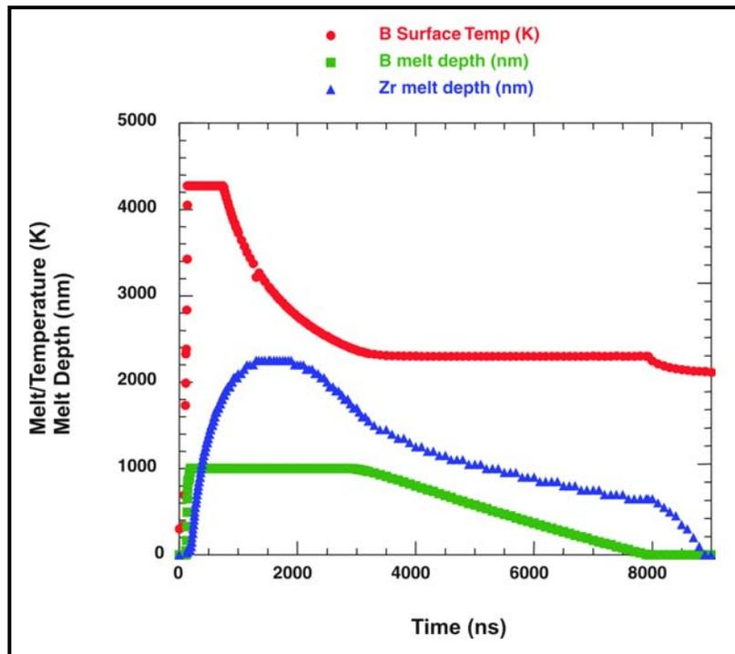
Figure 5. Numerical simulation of melting, liquid diffusion, and rapid solidification for a 1  $\mu\text{m}$  boron film sputter deposited on zirconium alloy.
