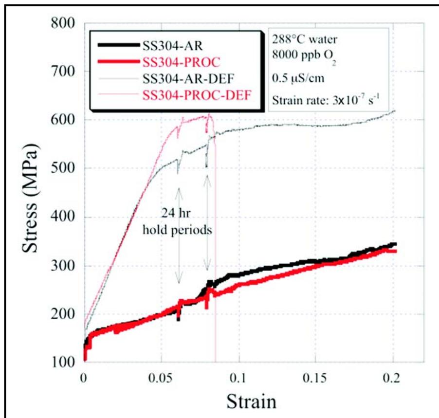
Figure 2. Stress-strain curves for the four SS304 samples tested.
