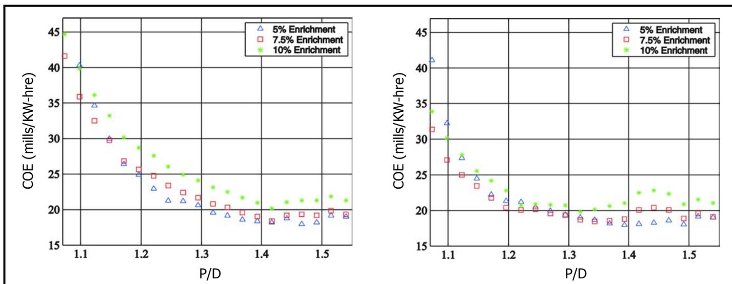
Figure 3. Minimum cost of electricity (COE) versus P/D for a major backfit scenario using  $UO_2$  fuel and coolant pressure drop of either 29 psia (left) or 60 psia (right).
