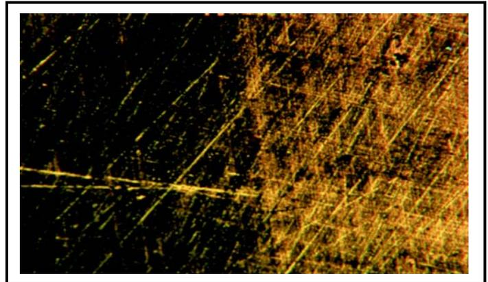
Figure 3. Synergistic effects of erosion and corrosion on  $C^+$  ion implanted Inconel 718 alloy after exposure to supercritical water at 500°C for 7 days. Left side of the sample was the non-reflective oxide deposit (thicker) and the right side showed a reflective metallic surface (thinner). SEM examination showed that the oxide particulates on the region with a metallic appearance were considerably less dense.
