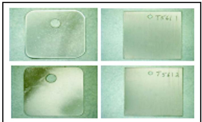
Figure 3. Surface of zirconium samples after autoclave testing at 800°F for 3 days (a) boron IBEST treated sample after sputter deposition with 0.75 μm boron layer and (b) control zirconium samples.
