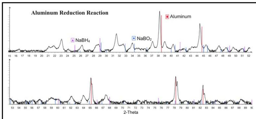
Figure 8. X-ray diffraction analysis for the Al and borate reaction.
