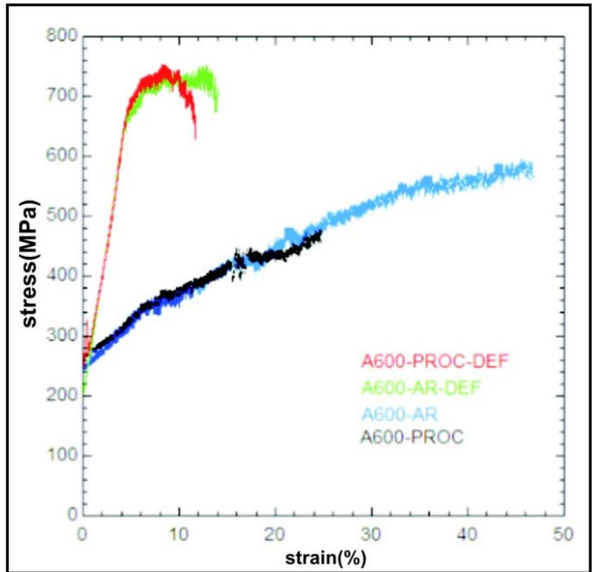
Figure 3. Constitutive response of Alloy 600 in 360°C primary water at a strain rate of  $3 \times 10^{-7} \text{ s}^{-1}$ .
