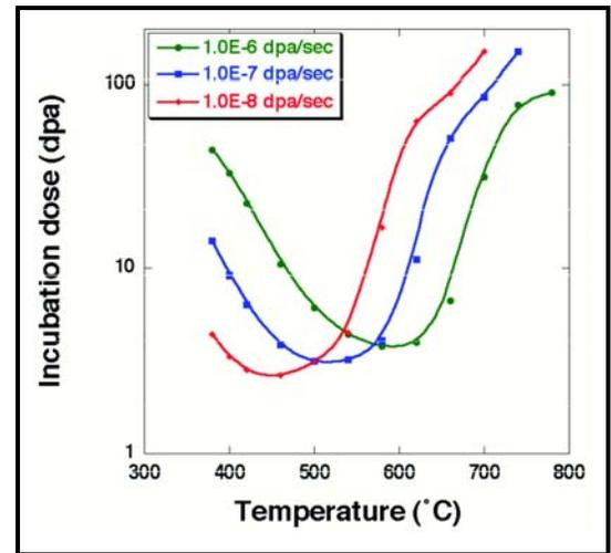
Figure 3. Incubation dose for void swelling in pure ternary austenitic steels as a function of irradiation temperature and dose rate.
