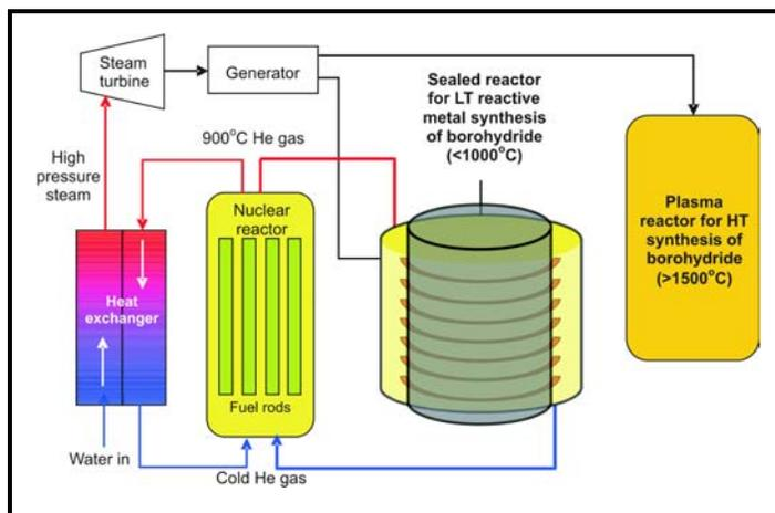
Figure 9. New concept using the gas-cooled reactor to produce hydrogen carrier materials.
