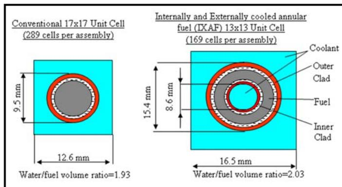
Figure 1. Annular fuel geometry compared to conventional solid PWR fuel.
