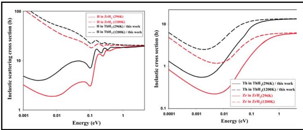
Figure 2. Inelastic scattering cross section of H, Th, and Zr in  $\text{ThH}_2$  and  $\text{ZrH}_2$ .
