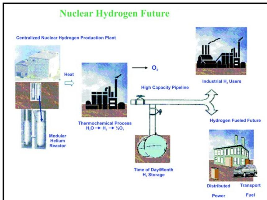
Figure 1. Schematic of a nuclear hydrogen future.
