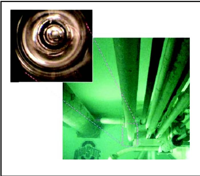
Figure 2. Scintillator disk located at the distal end of a titanium light guide, near the core of The Ohio State University Research Reactor operating at 1 kW.
