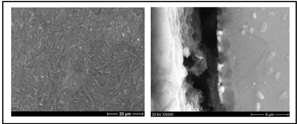
Figure 1. Surface of a zirconium alloy deposited with a 0.75 μm film of boron and IBEST treated with an ion energy range of 4-6 kJ/cm<sup>2</sup>, (a) surface view and (b) cross-sectional view where arrows indicate the boron alloyed layer.
