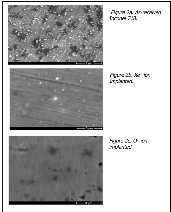
Figure 2. Nucleation of oxide on Inconel 718 after exposure to supercritical water at 300°C for 7 days: (a) as-received, (b)  $Xe^+$  ion implanted, and (c)  $O^+$  ion implanted.
