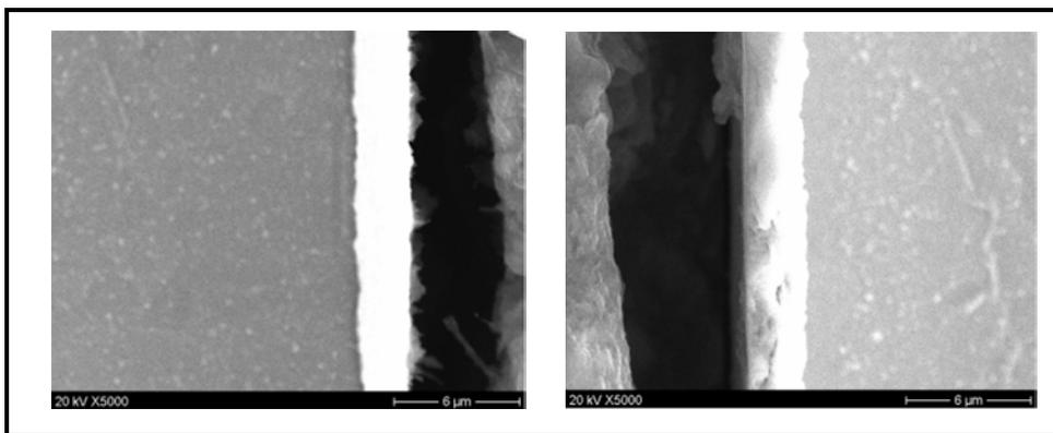
Figure 4. Cross-sectional SEM micrograph showing a nearly identical build-up of the oxide corrosion product on zirconium-alloy samples after autoclave testing for (a) control sample and (b) boron IBEST treated samples after sputter deposition with 0.75  $\mu\text{m}$  boron layer.
