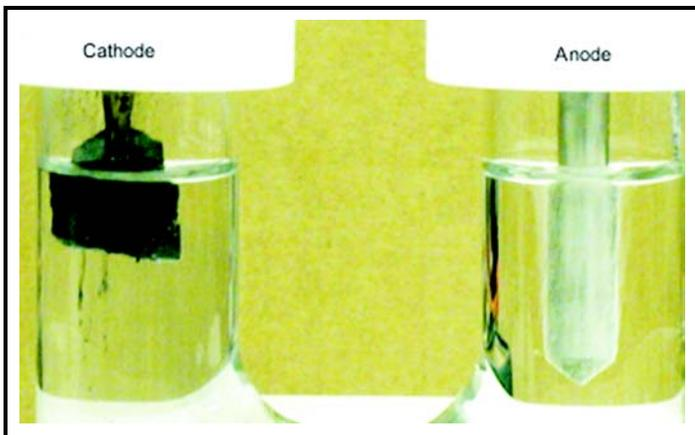
Figure 1. Test of tellurium as cathode for hydrogen generation suppression.
