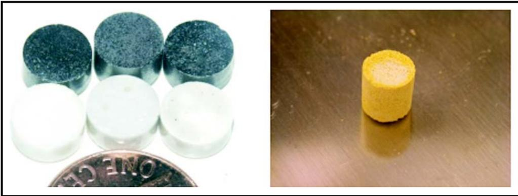
Figure 2. Photograph of co-sintered  $\text{UO}_2$  - BeO (black) & BeO (white) pellets (left). BeO ‘skeleton’ obtained by chemical dissolution of  $\text{UO}_2$  from a co-sintered pellet (right). The skeleton was about 85 percent dense and absence of  $\text{UO}_2$  was confirmed via EDS & XRD analysis.
