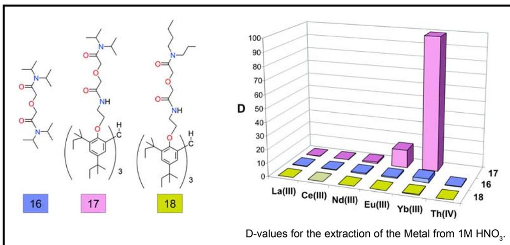
Figure 2. Extraction properties of the diamide ligands developed at University of Florida.
