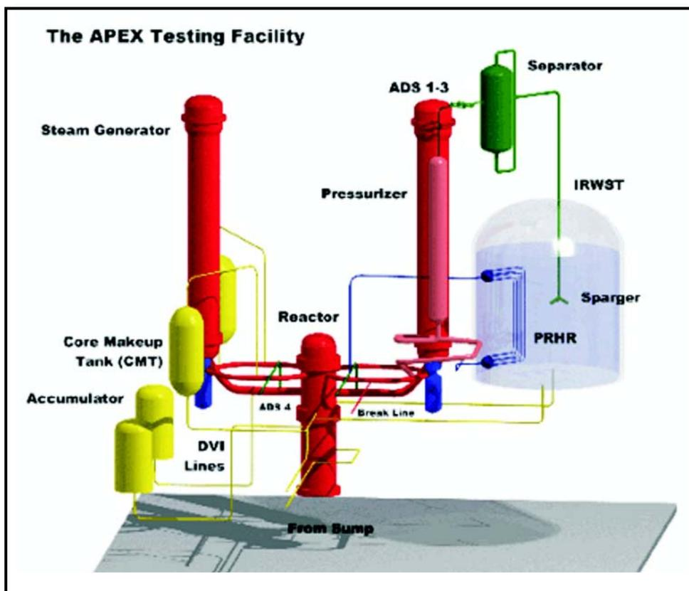
Figure 1. APEX-1000 integral system test facility at OSU.
