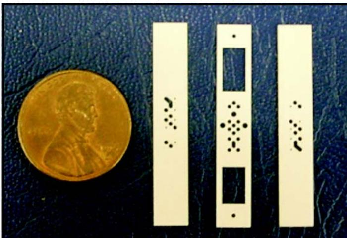
Figure 4. Alumina substrates for final (third) generation of MPFDs, showing the cavity and base pieces that form the detector.
