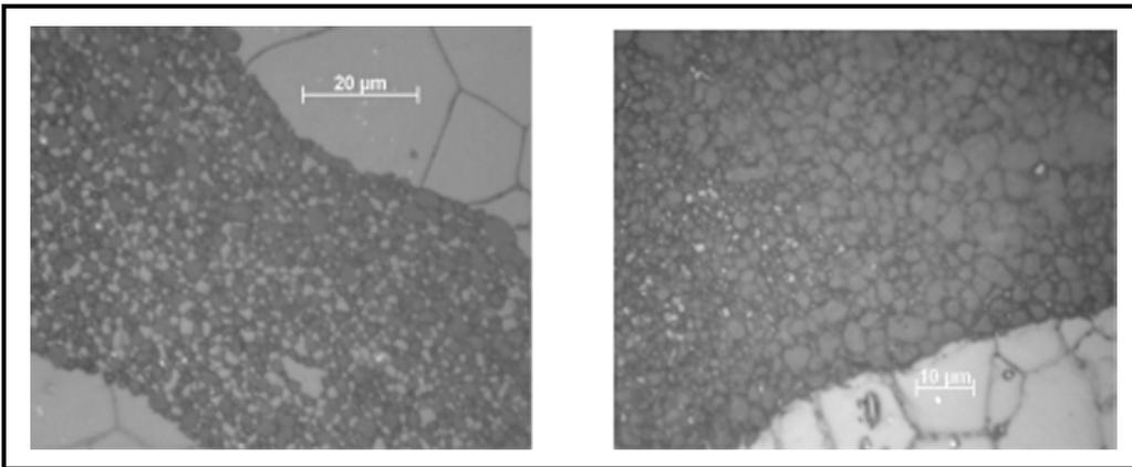
Figure 3. Polished, thermally etched section of a co-sintered  $\text{UO}_2$  - BeO pellet fabricated from green granules (left), and from bisque granules (right). Light regions correspond to the  $\text{UO}_2$  phase, while the grey regions correspond to the BeO phase. Reduction in the amount of dispersed  $\text{UO}_2$  phase within the BeO phase from the green to bisque granules is apparent.
