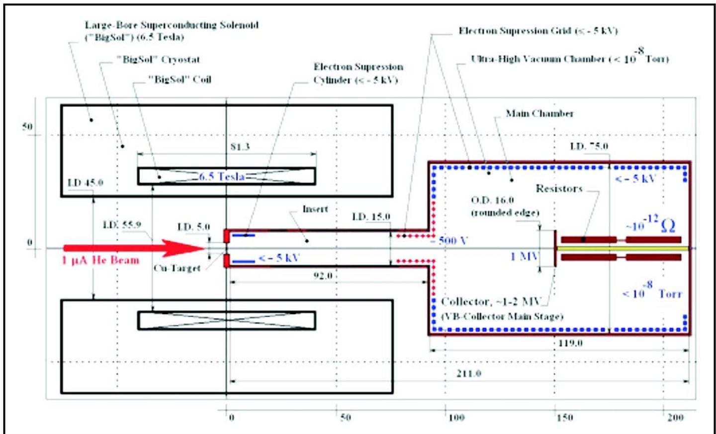
Figure 2. Component layout and main design parameters of the FFMC prototype.
