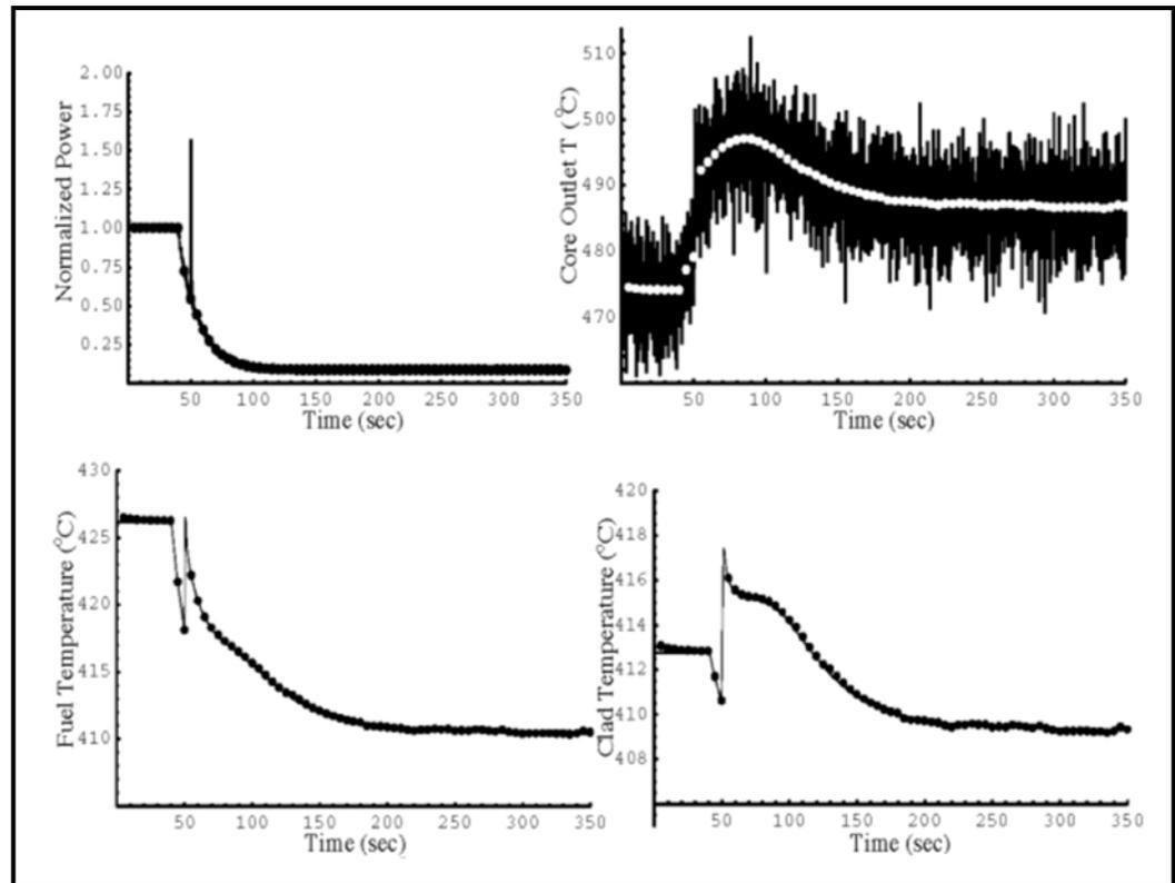
Figure 1. Reactor power, core outlet, fuel and clad temperature state estimates (dots) compared to true or measured system values (lines). Note that measured values include significant noise but state estimates are smooth.
