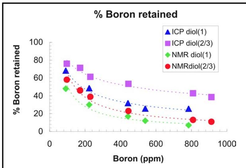
Figure 3. Percentage of total boron retained as measured by extraction experiments and as measured by  $^{11}\text{B}$  NMR. Extraction data: diol fully functionalized ( $\blacktriangle$ ), diol 2/3 functionalized ( $\blacksquare$ ).  $^{11}\text{B}$  NMR data: diol fully functionalized ( $\blacklozenge$ ), diol 2/3 functionalized ( $\bullet$ ).
