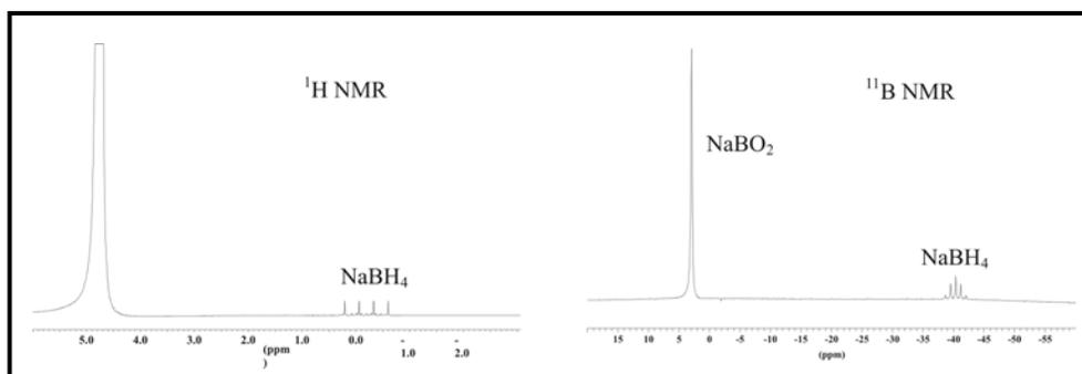
Figure 6. NRM confirmation of sodium borohydride synthesis in thermal plasma.
