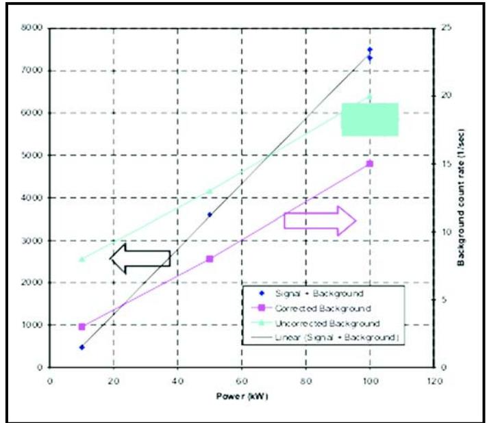
Figure 3. Reactor power versus measured photon count rate.
