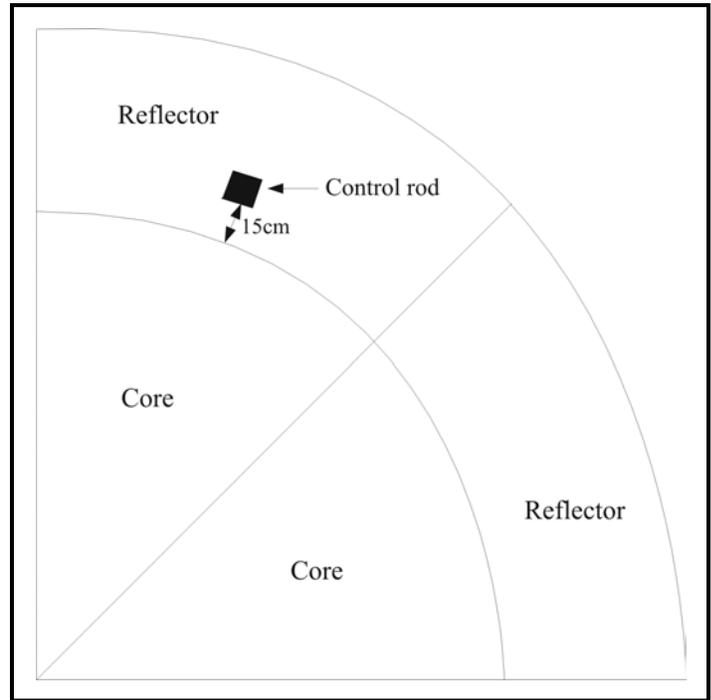
Figure 1. Two-dimensional PBR benchmark configuration.
