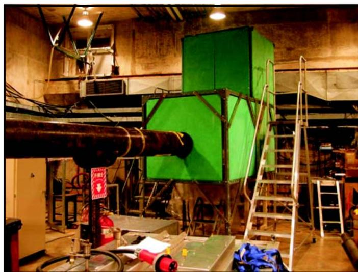
Figure 6. The assembled experimental system showing the polyethylene shielding structure surrounding the graphite heating system.
