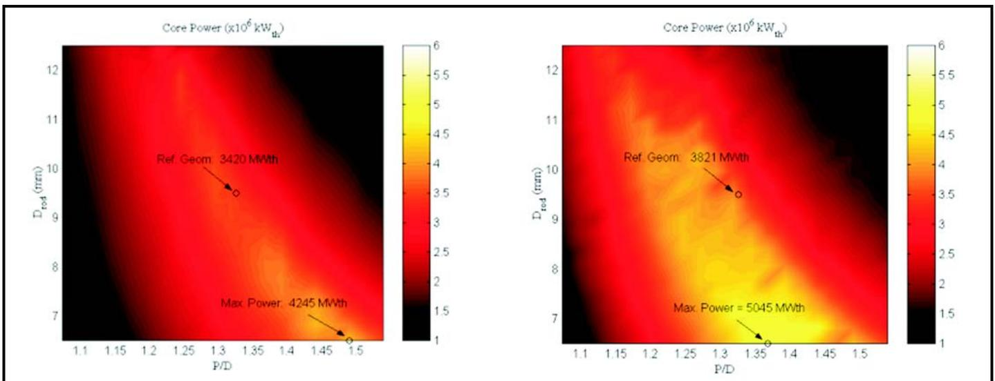
Figure 2. Attainable power from cores having different combinations of D and P/D in a square array of UO<sub>2</sub> fuel with a coolant pressure drop of 29 psia (left) or 60 psia (right).
