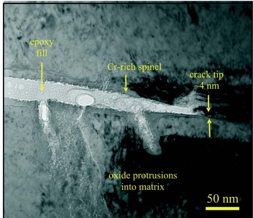
Figure 1. Crack tip in a 304SS crack-growth sample after test in oxidizing water at 288°C. Intergranular cracks decrease in width from >100 nm to ~4 nm at the tip.
