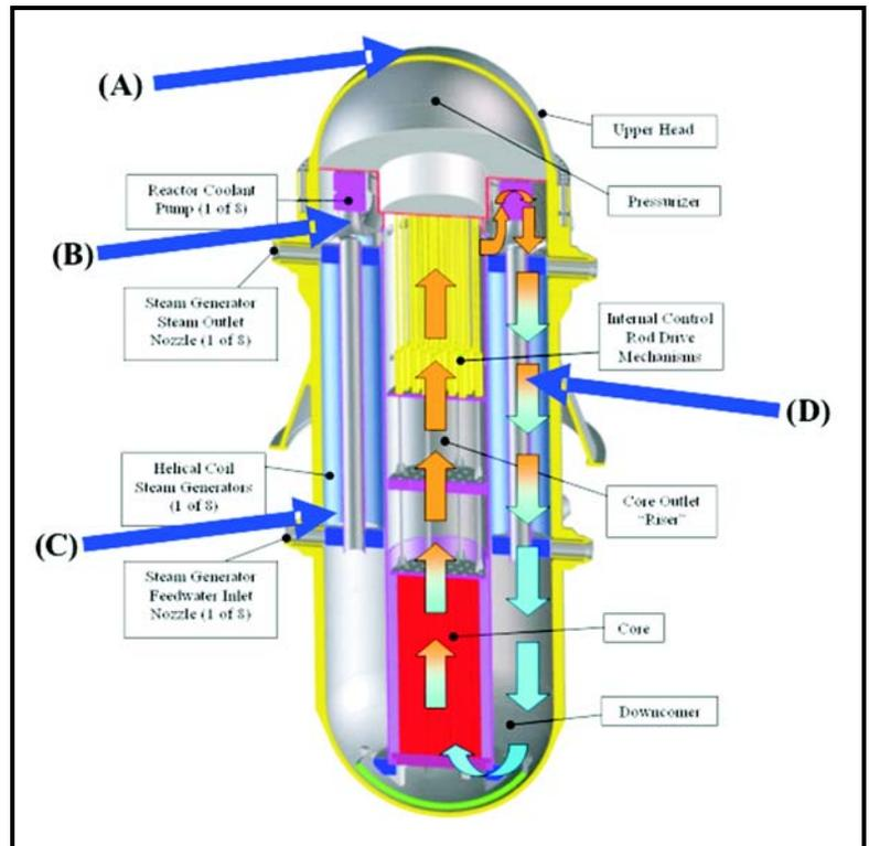
Figure 1. Components inside integral reactor pressure vessel and potential areas for on-line NDE: (A) upper head penetration welds, e.g., instrumentation tubes; (B) pump attachment; (C) steam generator tubes and tube attachment; and (D) primary coolant flow.
