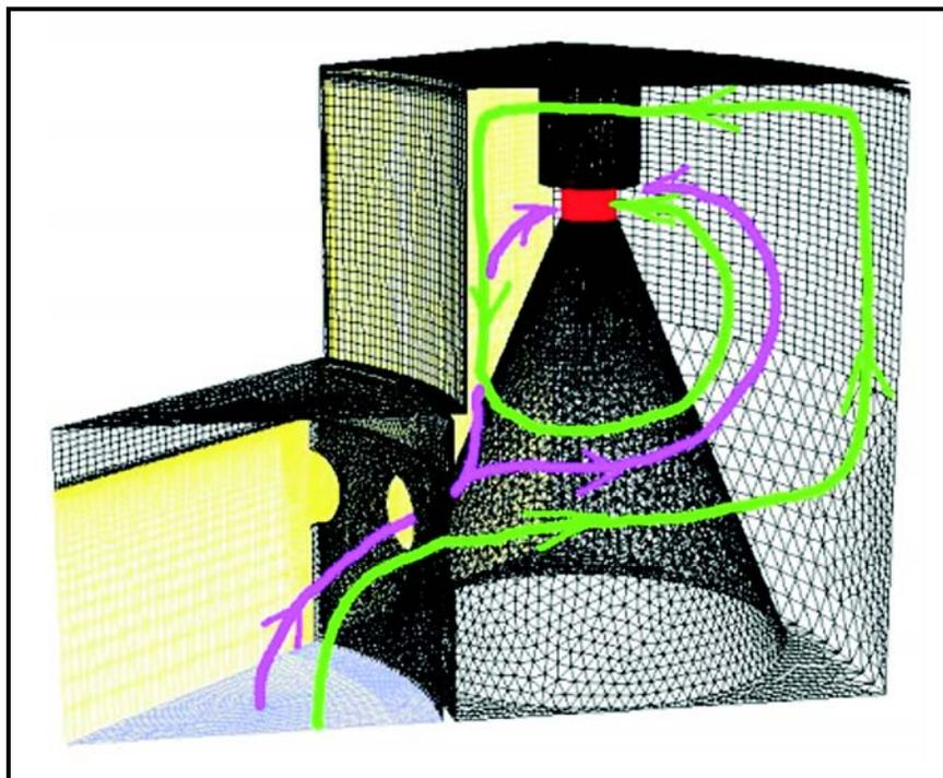
Figure 1. Pressurizer CFD model of pump plenum.
