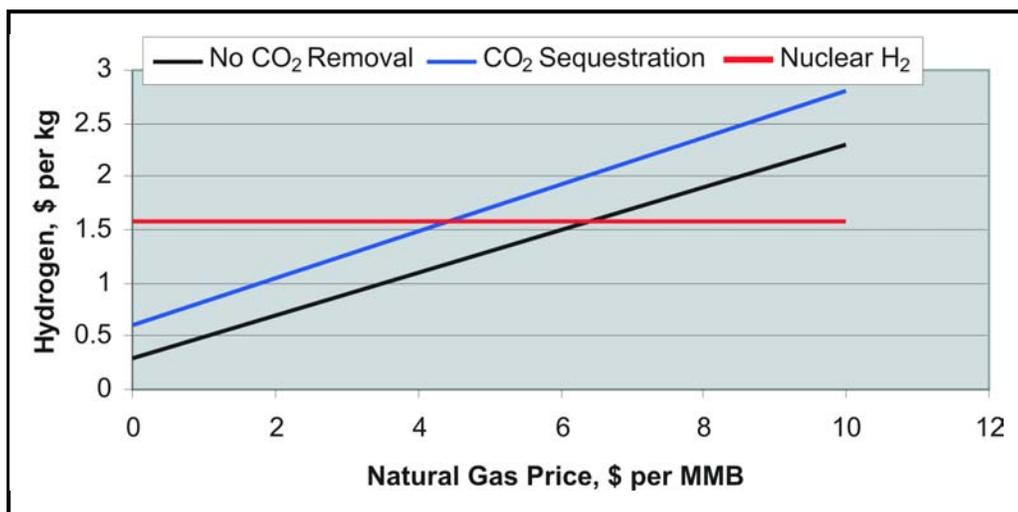
Figure 3. Nuclear hydrogen cost comparison with steam reforming.
