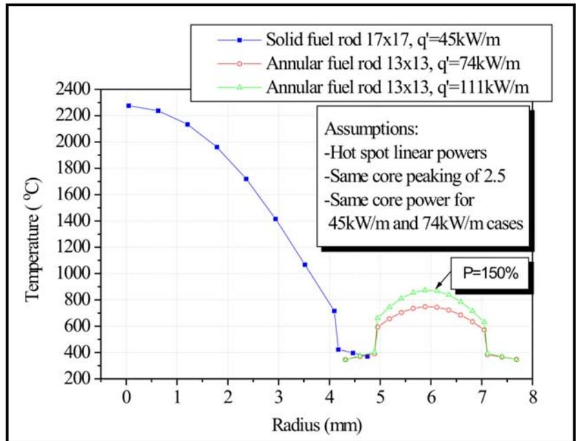
Figure 2. The graphic compares performance of solid and annular fuel.
