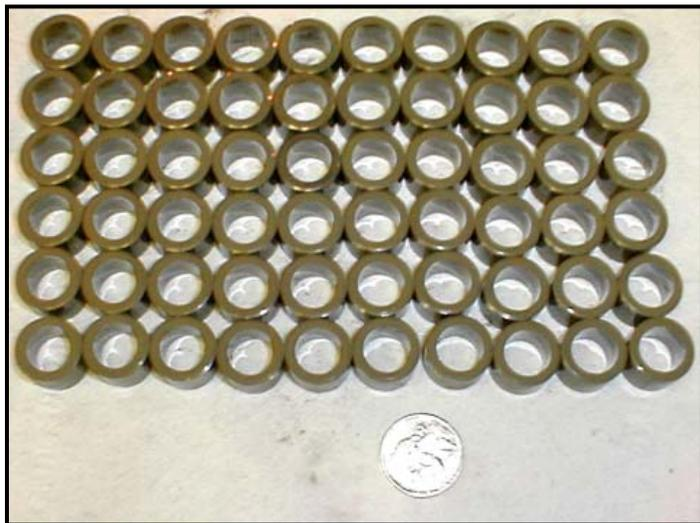
Figure 3. Sintered annular pellets manufactured at Westinghouse.
