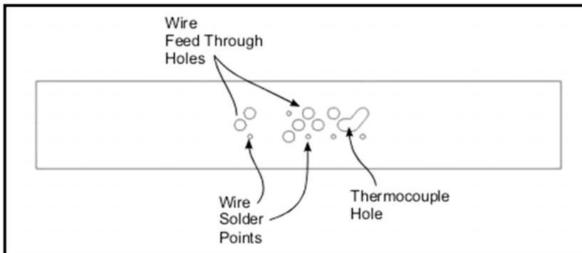
Figure 2. Aluminum oxide base (front view) showing the locations for feed through wires, wire attachment locations, and a temperature monitor (thermocouple).
