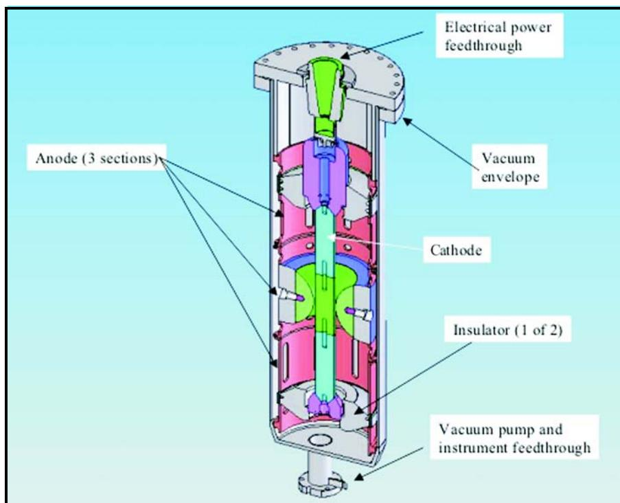
Figure 1. Final FEC prototype layout.
