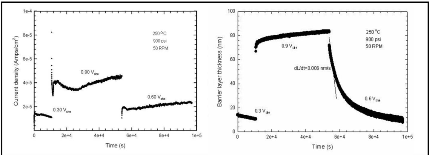
Figure 2. Experimental transients of current density and film thickness for the growth and thinning of the passive film on zirconium in 0.1M B(OH)<sub>3</sub> and 0.001M LiOH solution at 250°C and 900 psi upon stepping the potential from 0.30 V<sub>she</sub> → 0.90 V<sub>she</sub> → 0.60 V<sub>she</sub>. (a) current density, (b) thickness calculated from capacitance ( $f = 1$  kHz).
