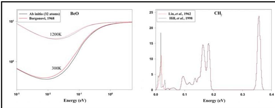
Figure 3. The thermal neutron scattering cross sections for  $\text{BeO}$  (left). The phonon spectrum of polyethylene (right).
