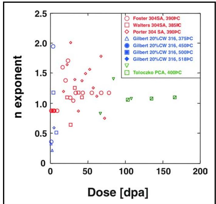
Figure 5. The exponent ( $n$ ) for the stress dependence of irradiation creep,  $\sigma^n$ .
