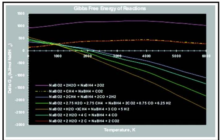
Figure 3. Gibbs free energy of reaction change for sodium borohydride synthesis.
