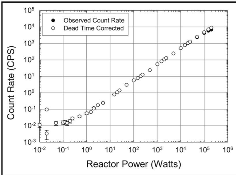
Figure 1. MPFD count rate as a function of reactor power.
