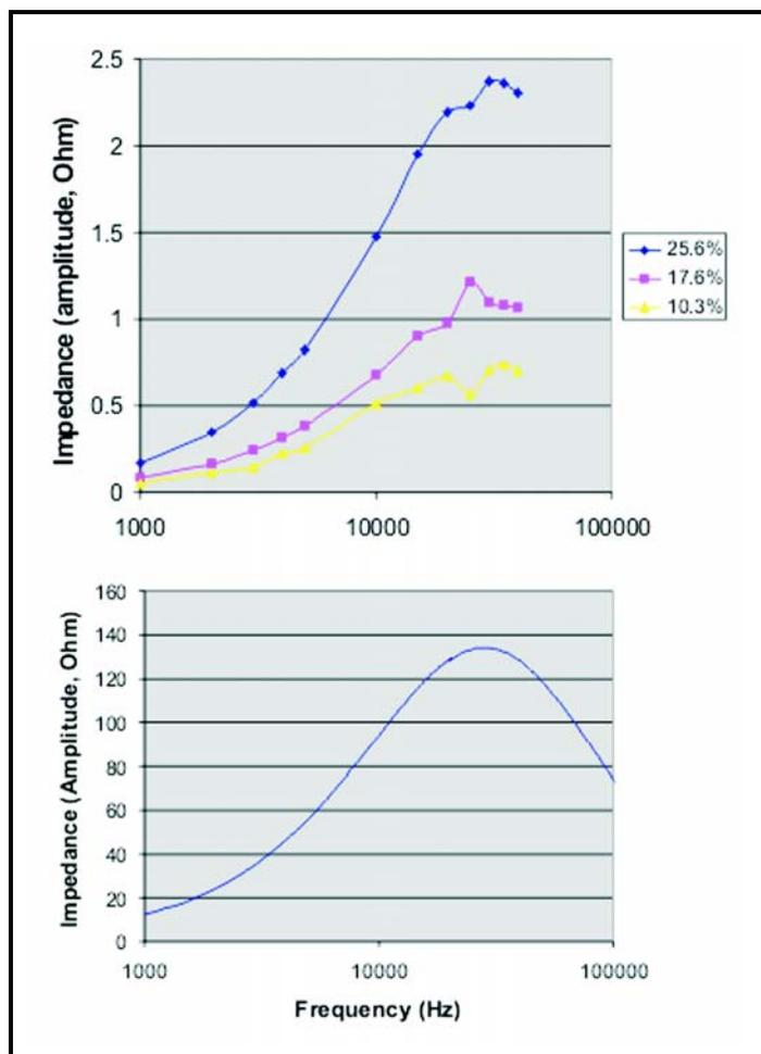
Figure 3. Experimental vs. computational EC deposit signals that peak at the 20-30 kHz range.
