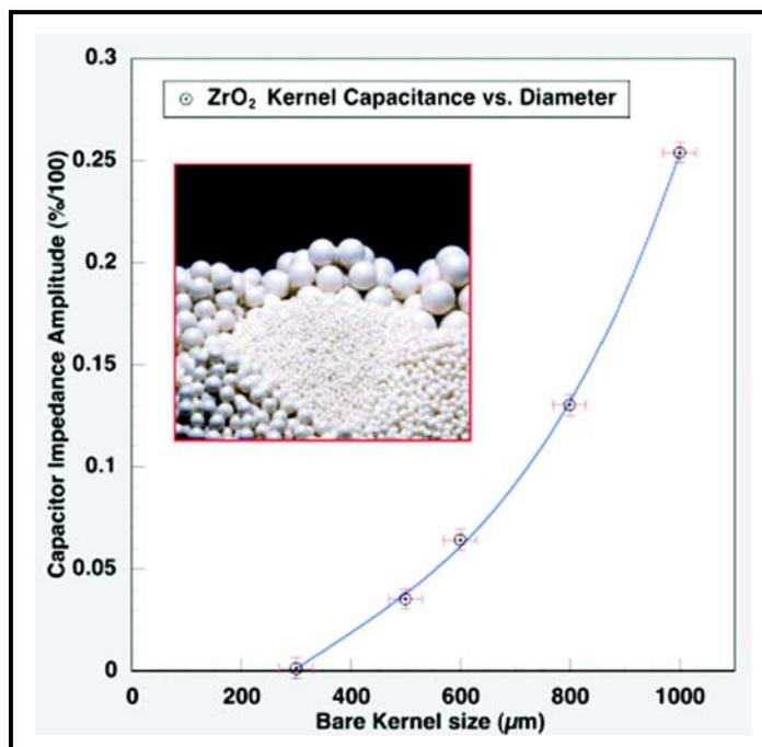
Figure 5. Capacitive sensor impedance amplitude vs. kernel diameter.
