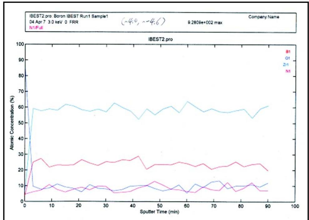
Figure 2. Auger composition vs. depth (sputter time) analysis showed uniform coexistence of boron and zirconium (at about 25 atomic percent boron).
