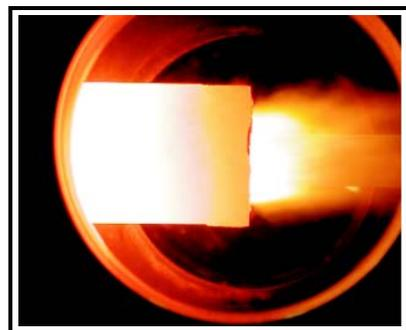
Figure 4. Thermal plasma synthesis of sodium borohydride.
