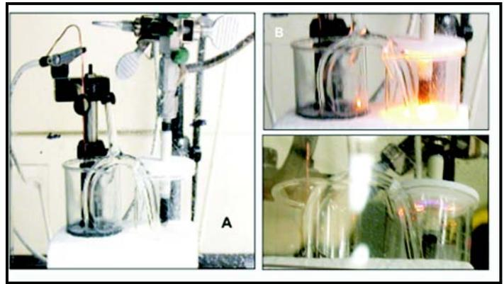
Figure 2. Salt bridge connected half-cells for plasma electrolysis experiments.
