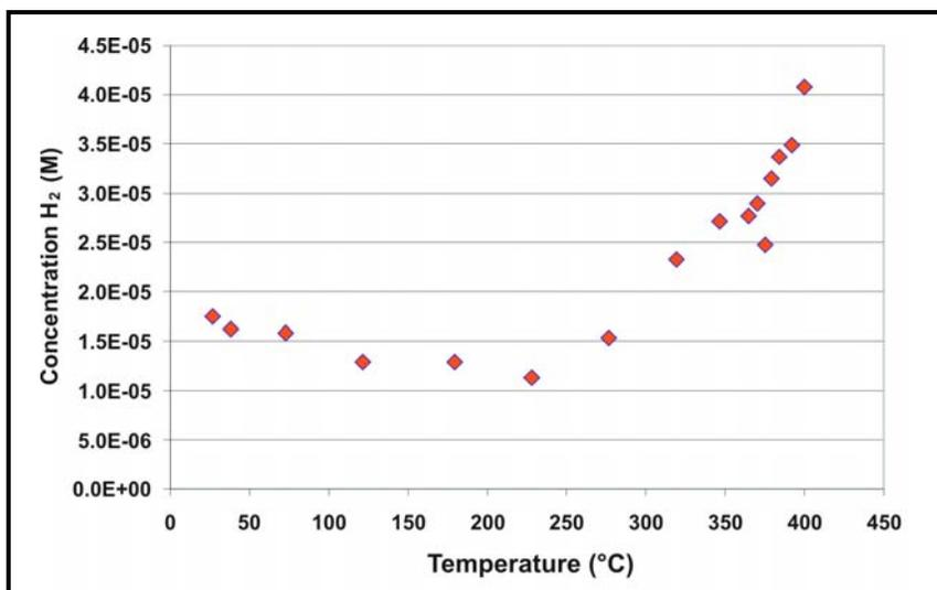
Figure 1. The concentration of  $H_2$  measured in the  $N_2$  saturated solution as a function of temperature at 250 bar pressure.
