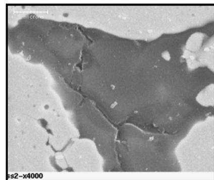
Figure 1. SiC phase (dark) within the open porosity of  $\text{UO}_2$  produced by Polymer Impregnation and Pyrolysis.
