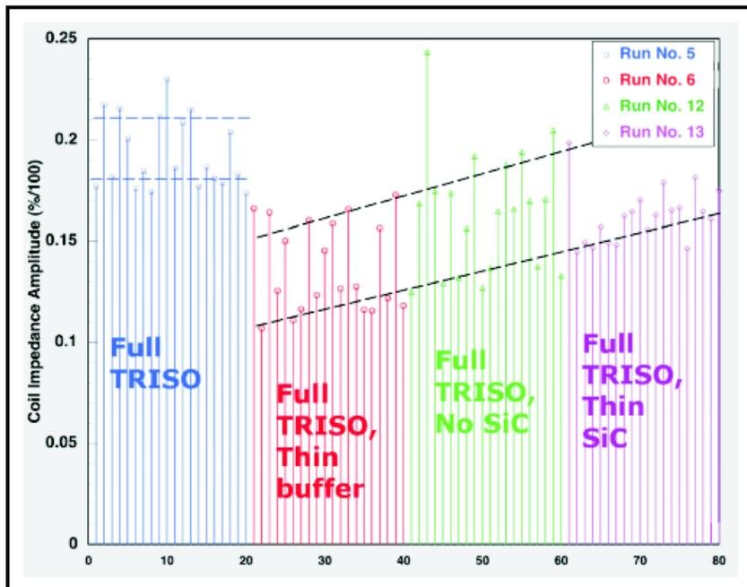
Figure 3. Induction coil measurements from randomly selected particles of four different coating conditions.
