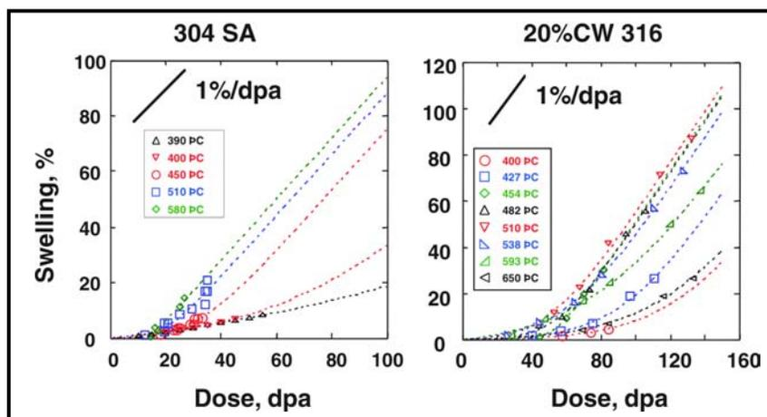
Figure 1. Swelling data for neutron irradiated solution-annealed 304 and for 20 percent cold-worked 316 stainless steels fitted to equation (2).
