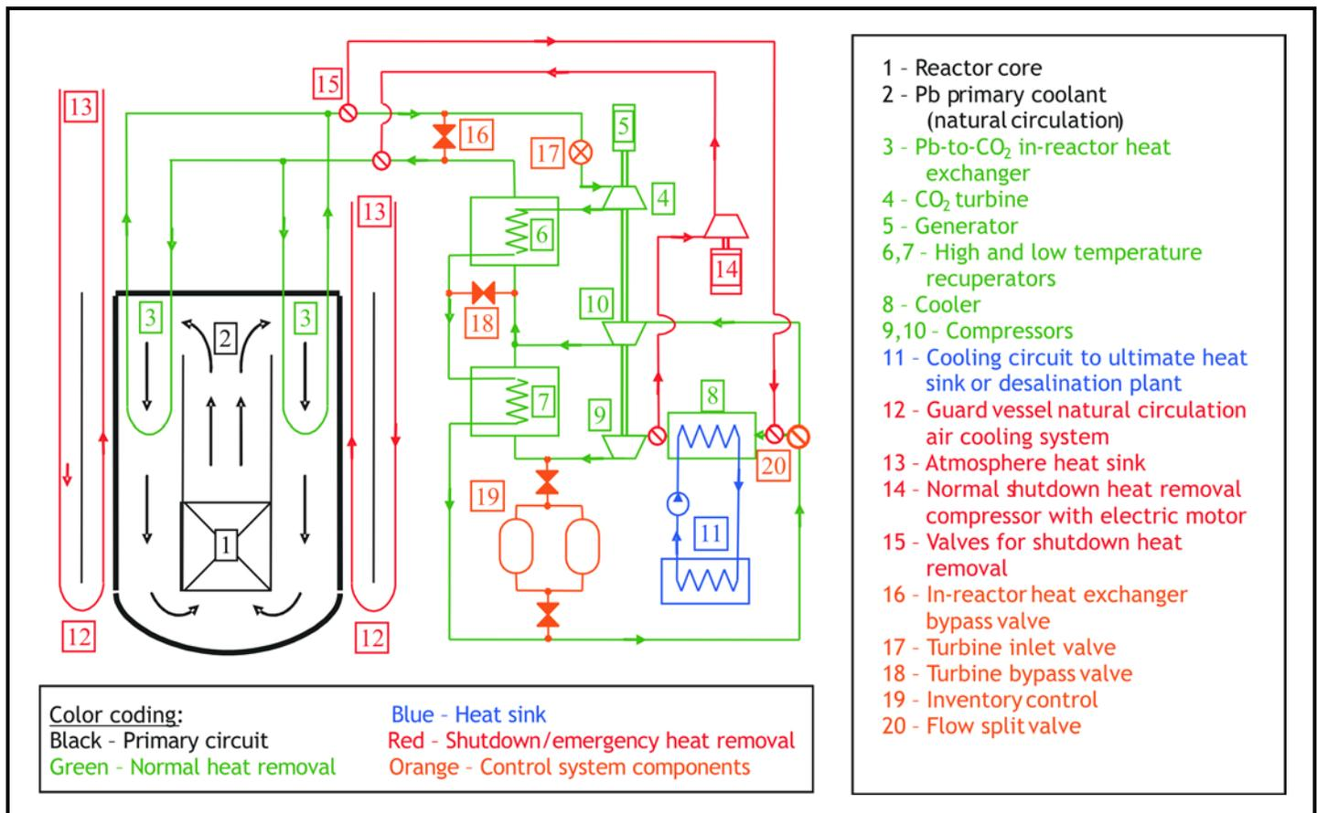
Figure 1. Schematic of coupled STAR-LM-S-CO<sub>2</sub> Brayton cycle nuclear power plant showing heat transfer paths and S-CO<sub>2</sub> Brayton cycle control mechanisms.
