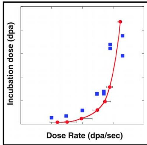
Figure 2. Computed vs. measured incubation dose for void swelling in pure ternary austenitic steels irradiated at about 400°C and at different dose rates.
