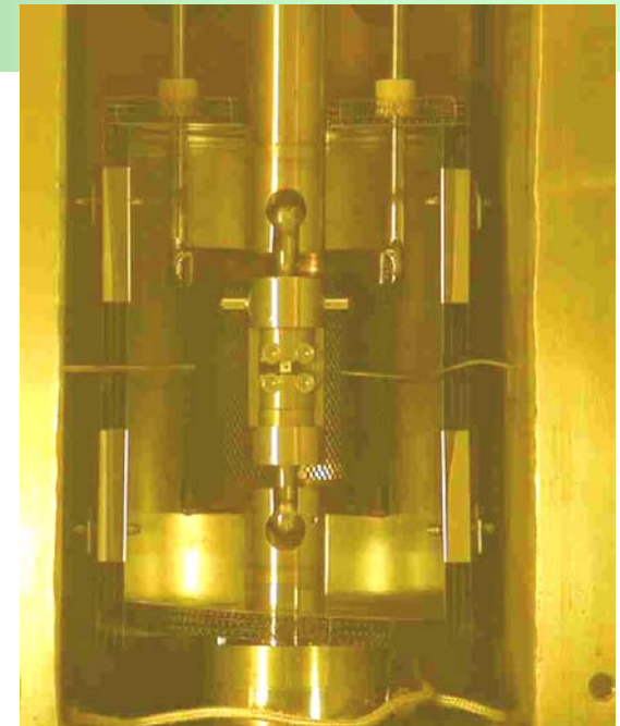
Tensile specimen testing apparatus in the CMR hot cell. Capable of testing at variable strain rates and temperatures up to 700°C
