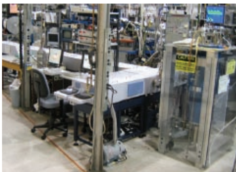
The Oxford Instruments magnet, installed next to the Bruker IFS 125HR spectrometer. The stainless steel tubes contain the optical coupling to the VUV-IR ring and between the spectrometer and the magnet.
