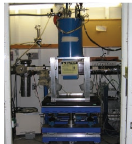
The magnet setup at X19A. It is mounted on an xyz table, which can be motor-controlled for ease of alignment. Samples are loaded from the top on a vertical rod into the sample space and are cooled by helium vapor or liquid from the magnet reservoir.
