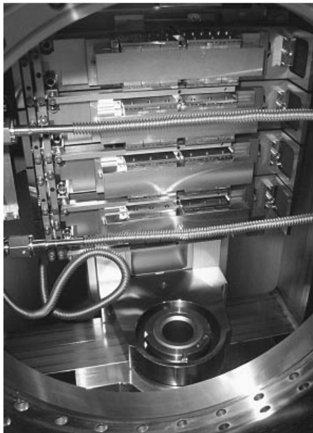
The new monochromator at beamline X1A1. It will provide for exchangeable gratings with higher diffraction efficiency, integrated water-cooling, and improved vacuum performance to minimize carbon contamination. It includes four selectable in-situ side-cooled grating holders, and provides for micro-radian angular precision and repeatability.
