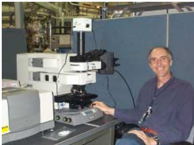
Figure 3: Gywn Williams (NSLS) at the helm of the new Spectra Tech Continuum infrared microscope with fluorescence microscopy capabilities.
