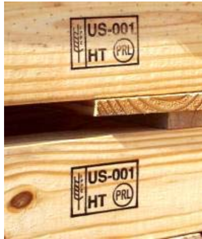
Figure 1. Marked pallets, the FAO logo, and the IPPC mark for wood packaging
