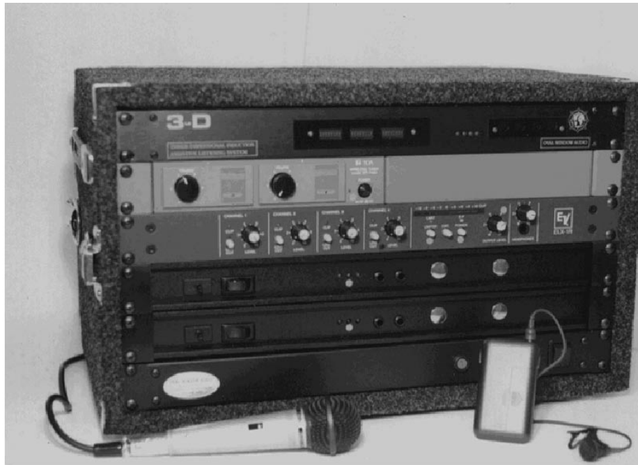
Figure 2. Oval window induction loop amplifier system , with wired and FM microphones
