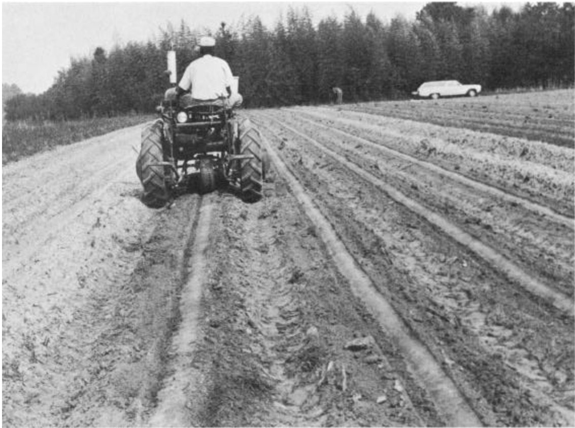
FIGURE 19.—Firm, moist seedbed developed by scraping off tops of ridges and placing seed, fertilizer, and weed-control chemical with planter with runner wings.
