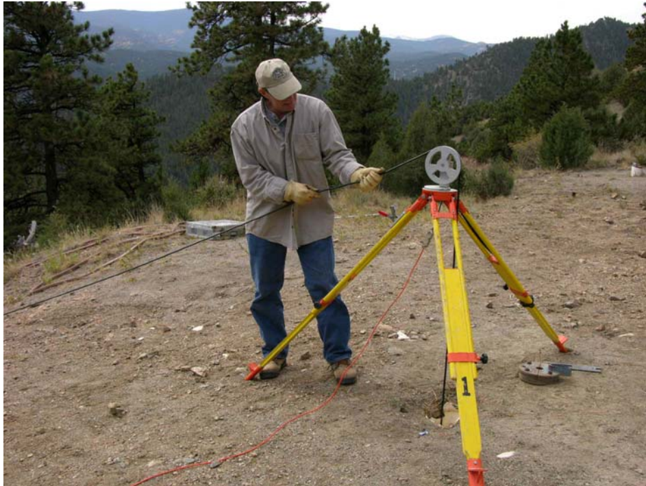
Figure 24. Performing hole-to-hole tomography by hand in the absence of the computer controlled winches and after depth encoder failure.
