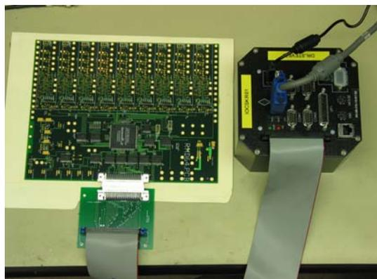
PCB electronics for testing commercial 3x3 Si APD array (contact: S. Ross)
