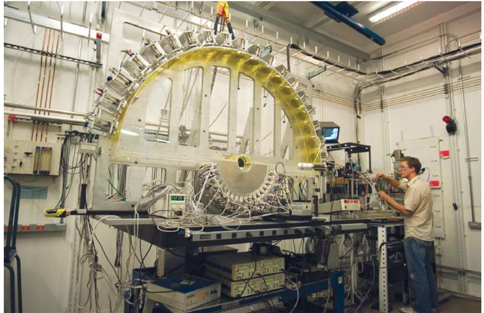
LERIX x-ray Raman scattering spectrometer at 20-ID, developed by G. Seidler and collaborators (T.T. Fister et al., "Multielement spectrometer for efficient measurement of the momentum transfer dependence of inelastic x-ray scattering," *Rev. Sci. Instrum.* **77**, 063901 (2006)).
