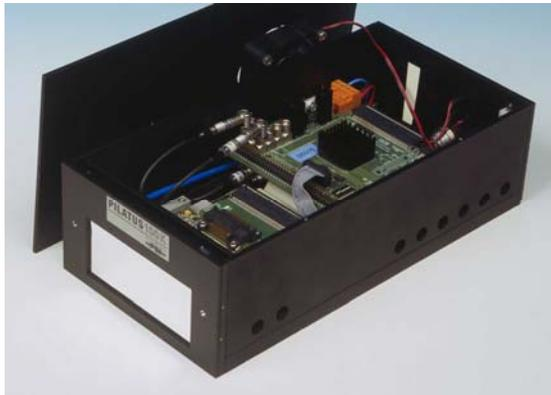
Pilatus 100K digital Si pixel array detector (SLS/PSI; XSD-BTS contact: A. Miceli)
