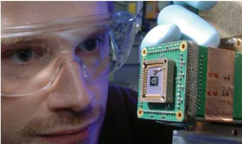
Detector for differential phase contrast imaging (S. Vogt, Sector 2), collaboration between APS-XSD X-ray Microscopy and Imaging Group and SUNY-SB/BNL.
