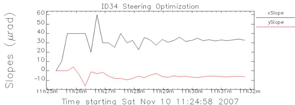
ID34 often requires a new steering of about 40  $\mu\text{rad}$  due to a beamline configuration change
