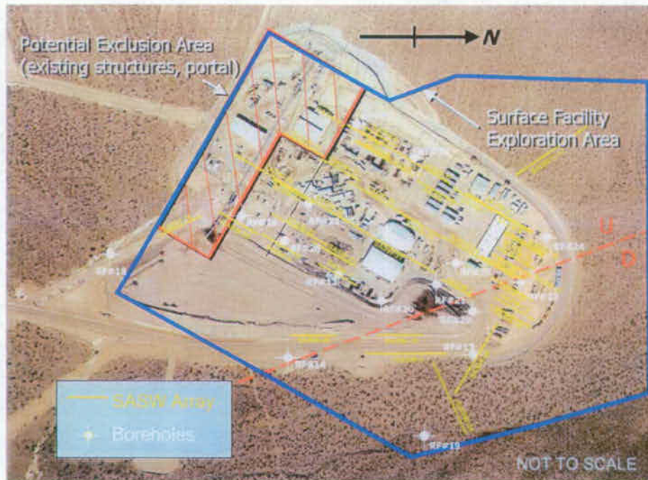
Figure 6-13. Locations of SASW lines at the surface facilities site [only pre-2004 lines shown]. (Figure 43 of BSC 2002a)
