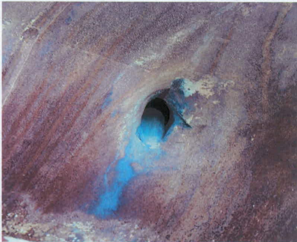
Figure 1.3. Puncture in Tank Car
