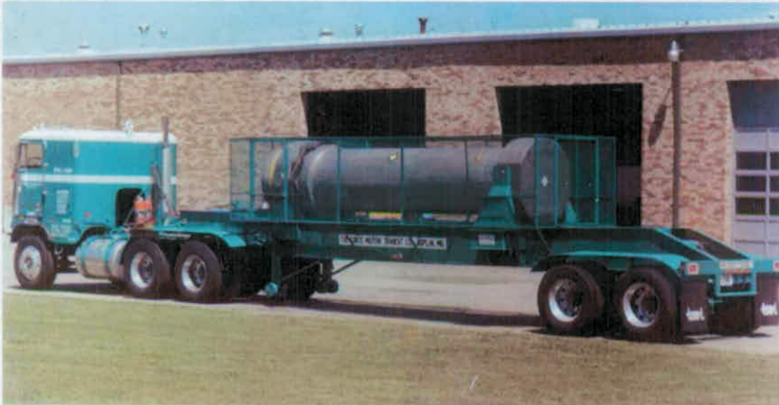
Figure 4.1. NAC LWT Transport Package (without ISO container)
