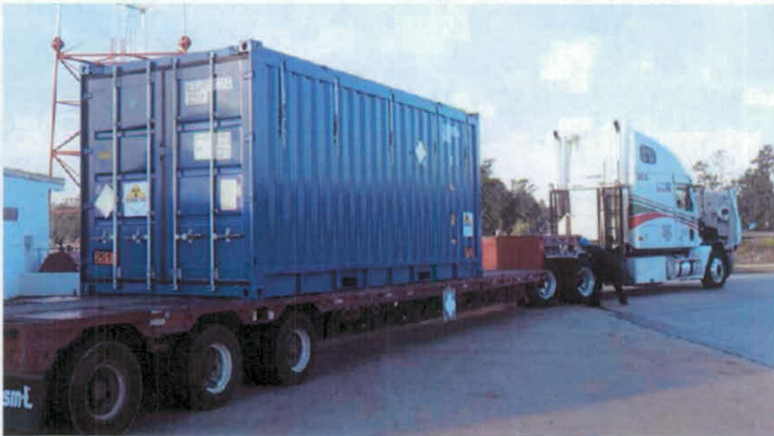
Figure 4.2. NAC LWT Transport Package (with ISO container)
