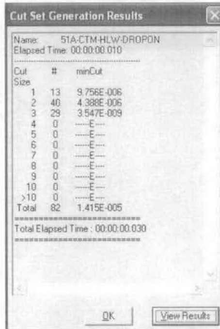
Figure B4.4-20 Uncertainty Results of the Drop of Object onto Canister Fault Tree
