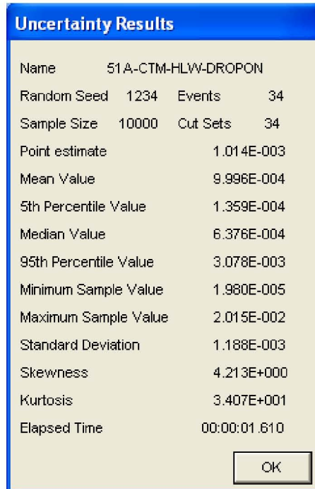
Figure B4.4-20 Uncertainty Results of the Drop of Object onto Canister Fault Tree
