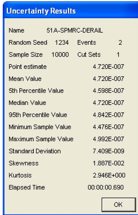
Figure B1.4-12. Uncertainty Results of the SPMRC Derailment Fault Tree
