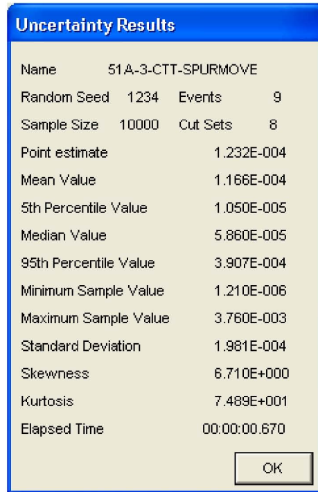
Figure B2.4-5. Uncertainty Results of the Spurious Movement of the CTT in the Cask Preparation Area During Cask Preparation
