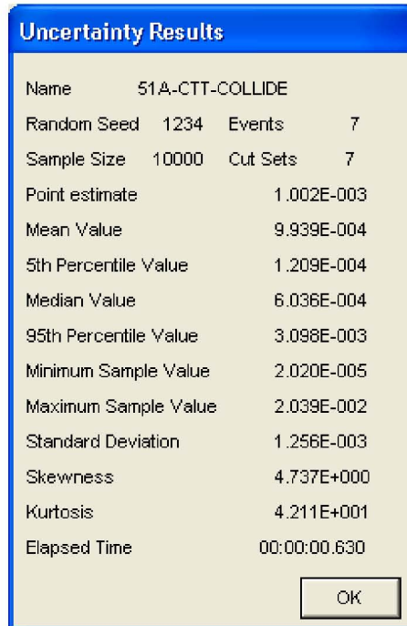
Figure B2.4-8. Uncertainty Results for the Collision of CTT during Cask Transfer Fault Tree
