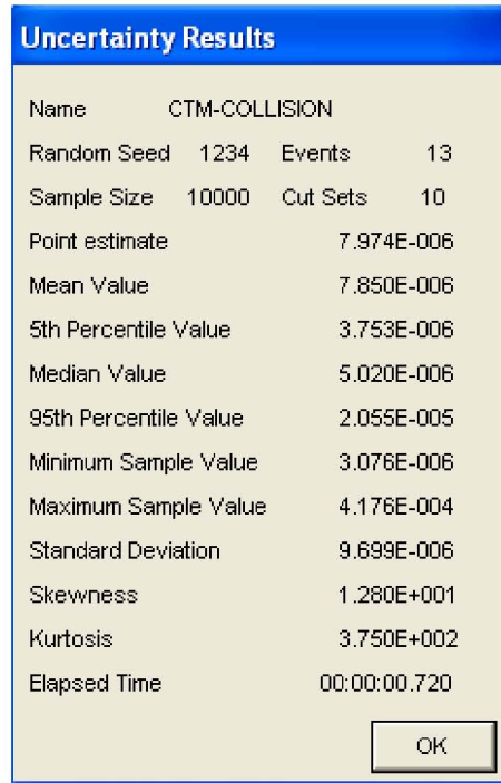
Figure B4.4-34 Uncertainty Results of the Canister Impact Fault Tree
