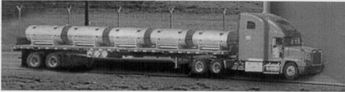
Figure C.1. Trailer carrying five UF 6 cylinders in overpacks (Photo courtesy of United States Enrichment Corporation [USEC 1999]).
