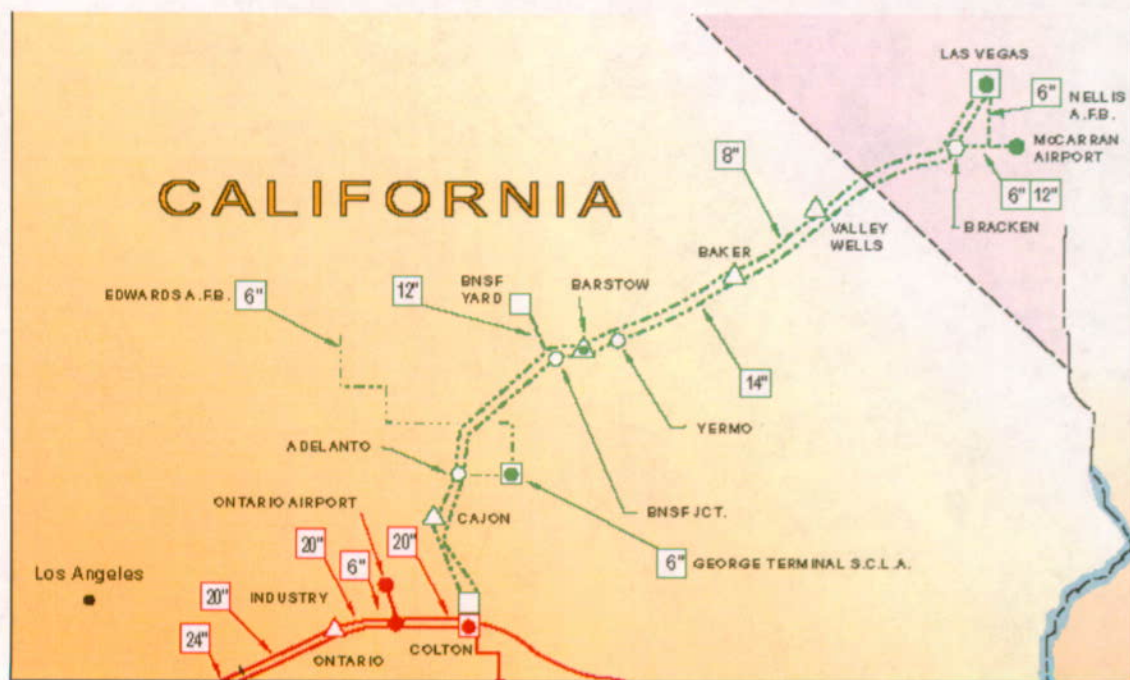
4-2 Figure Kinder Morgan, Inc. Colton to Las Vegas Pipeline System
