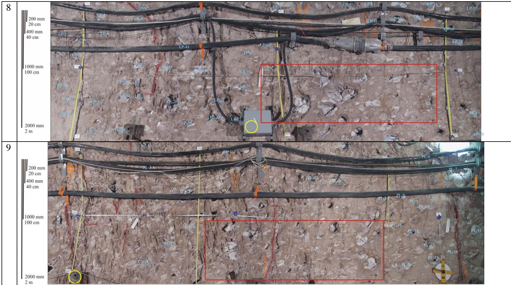
Figure A4-8. Panel Photograph at Station 18+05 on Left Wall and Small-Scale Fracture Traverse Location H7 with Vertical Traverses V19, V20, and V21 with Lithophysae Larger Than 20 cm in Diameter Inventoried for Shape and Panel Map 18+05L Location Indicated in Red Box (See Section A3)
