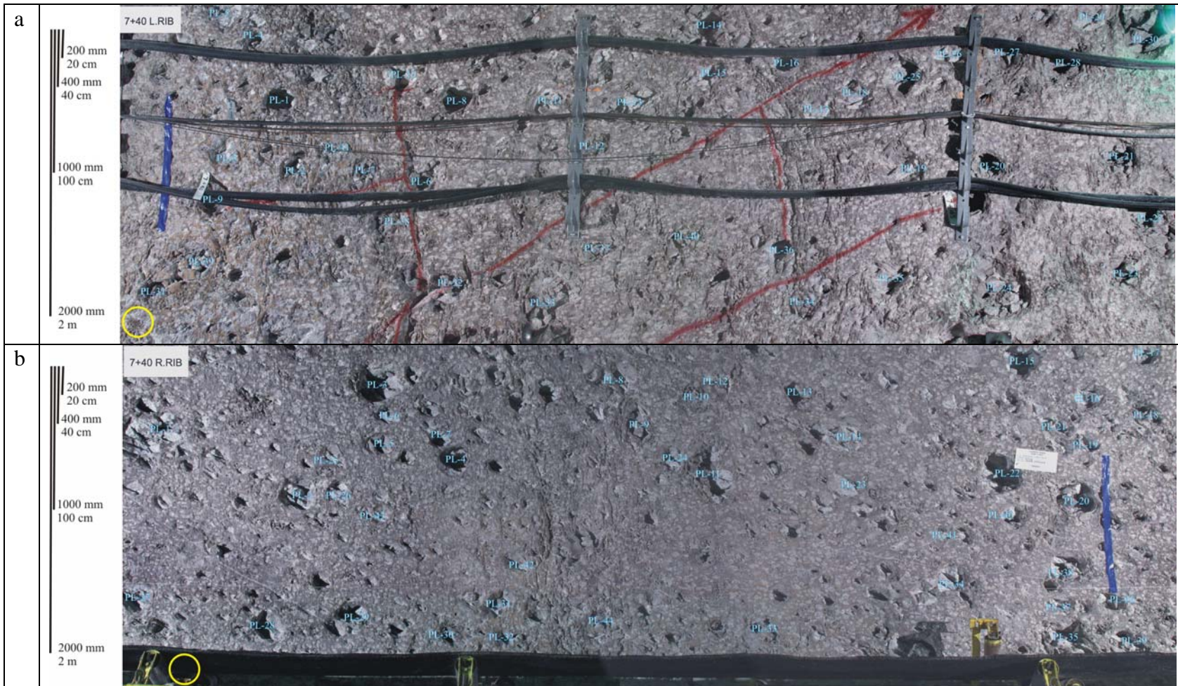
Figure A4-2a. Panel Photograph at Station 07+45 on Left Wall and Small-Scale Fracture Traverse Location H15 with Vertical Traverses V37, V41, and V42 with Lithophysae Larger Than 20 cm in Diameter Inventoried for Shape
