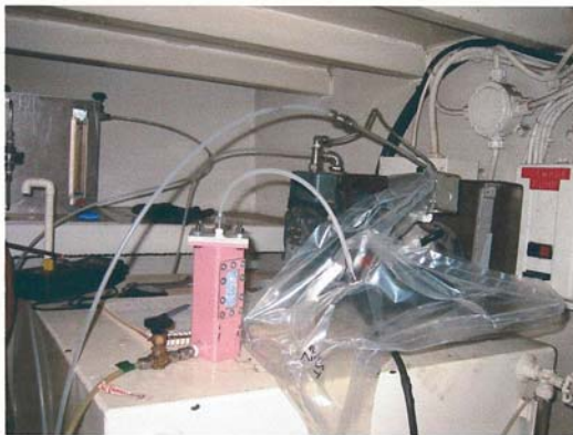
Filling Hydrocarbon test bag for lab test
