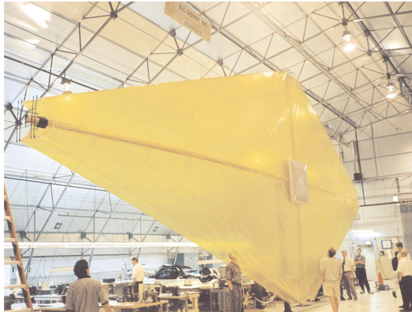
Figure 12.10. Half-scale NGST sunshade deployment demonstration at ILC Dover.
