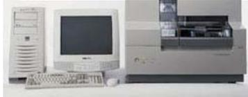
Multi-Color Capillary Electrophoresis
