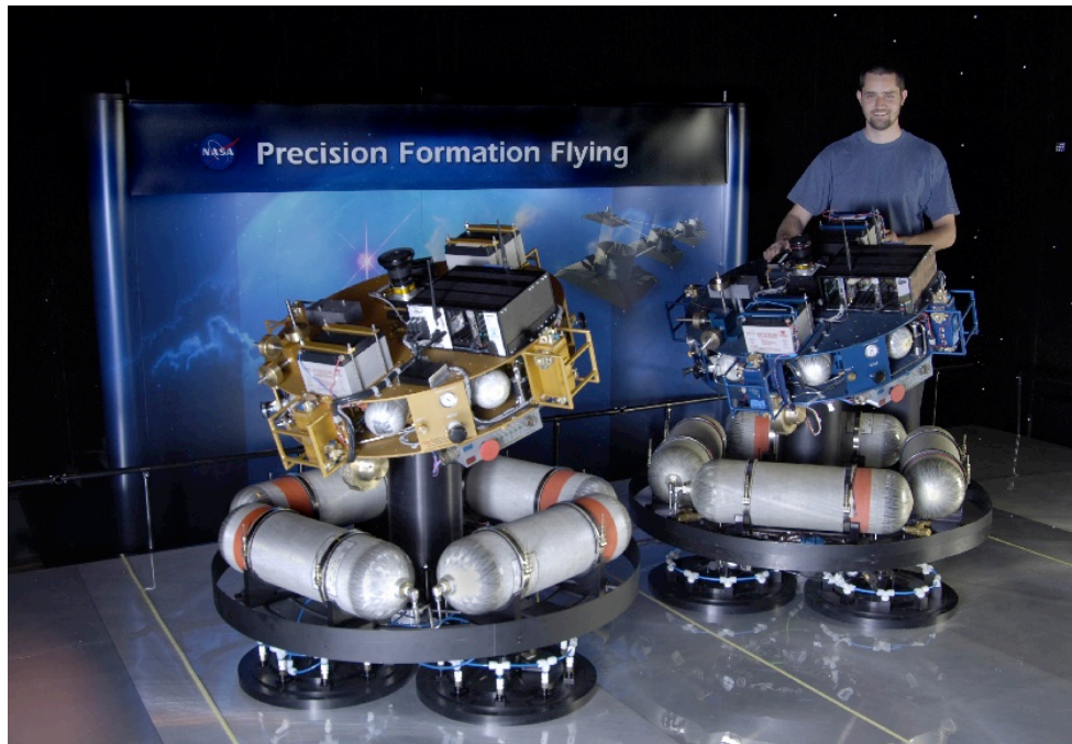
Figure 1: The Formation Control Testbed (FCT). Shown are the two robots on the flat floor with Jason Keim, the FCT Operations Lead. The floor is flat to 0.002 in., level to 120 \mu rad, and spans a 7.3 m x 8.5 m area. The robots’ attitude platforms (shown tilted for each robot) also float on spherical air bearings. As a result, the attitude platforms have extremely low-friction 5DOF motion. The final, vertical degree of freedom will be provided by retrofitted vertical stages that can translate 0.5 m. The robots serve as the system-level testing ground for flight software developed for space applications in formation flying.
