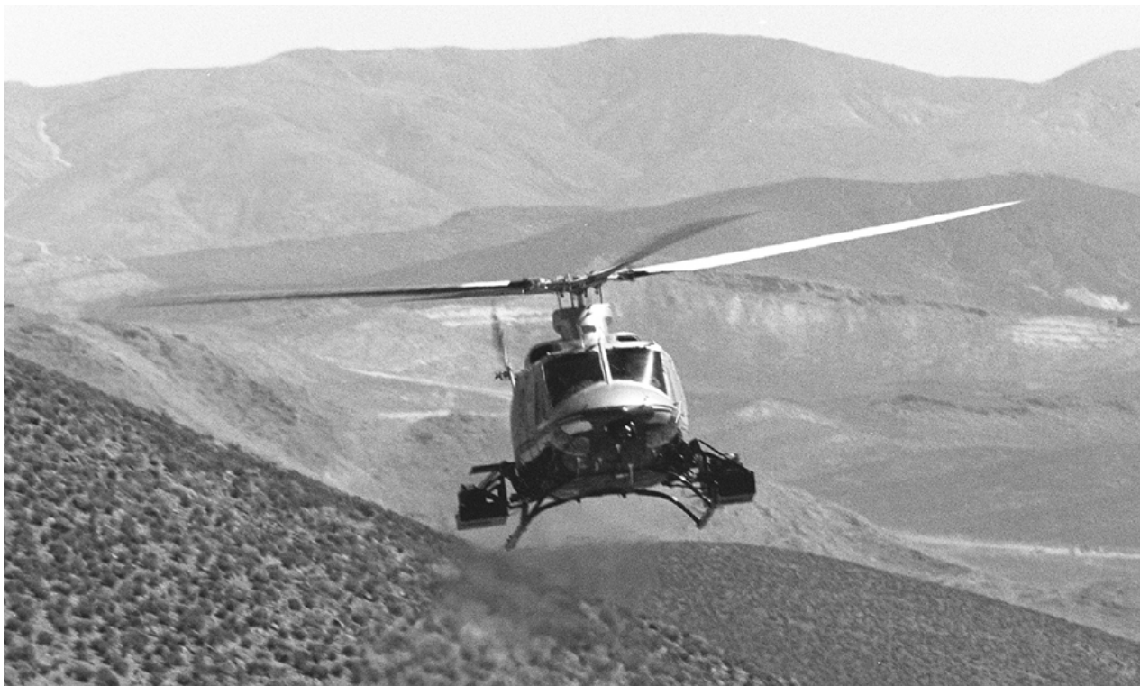
Figure 3: Aerial Measuring System Aircraft With Detection Equipment
