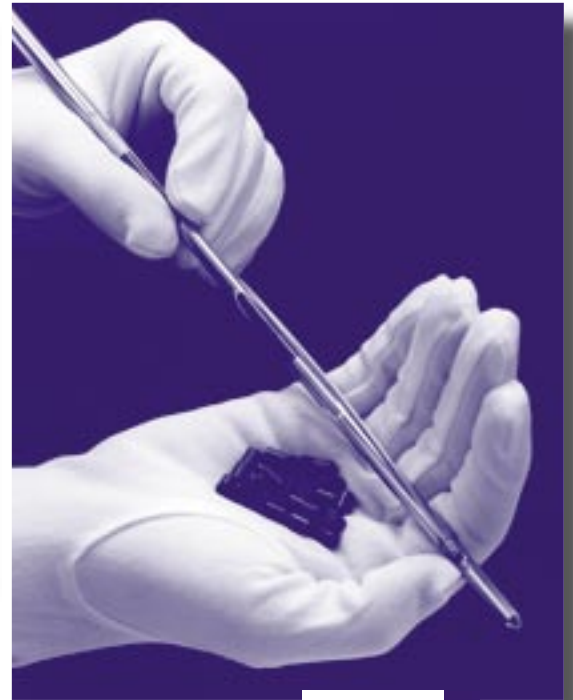
Spent nuclear fuel is most commonly in solid ceramic pellet form, about the size of a pencil eraser, secured inside an assembly of strong metal tubes.
