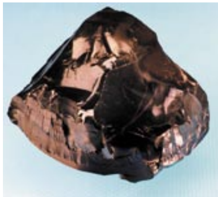
High-level radioactive waste is made solid by mixing it with glass-forming chemicals in stainless steel canisters and then subjecting it to heat. The result is a hard glass-like substance.
