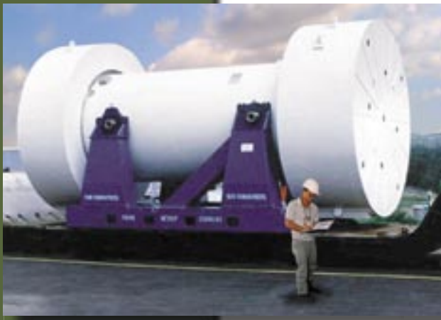
Rail cask with impact limiters designed for the transportation of spent nuclear fuel and high-level radioactive waste.
