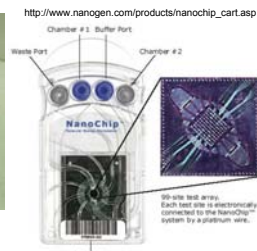
NanoChip™ from Nanogen (Miniature Bioassay Device)
