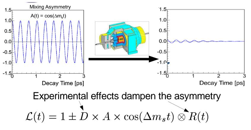
•A is know as the Amplitude: the size of the asymmetry, corrected for detector effects.
