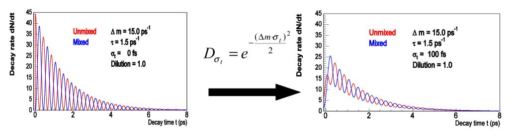
Smearing of decay time causes attenuation of asymmetry signal:
