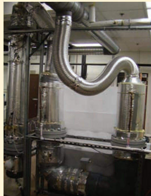
Pictorial view of the laboratory-scale diffusion driven desalination experiment
