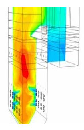
Evaluate boiler combustion modifications for combined NOx and mercury control
