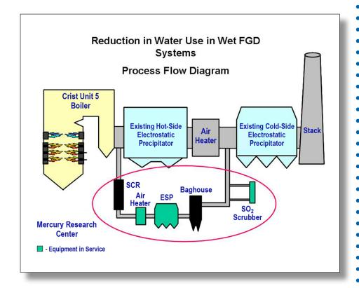
The process at Plant Crist includes air pollution control devices that may be more effective at lower flue gas temperatures.
