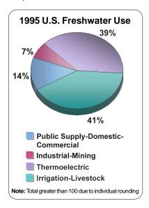
In 1995, fossil-fuel-based thermoelectric generators were second only to agriculture in total freshwater withdrawals. In that year, which represents the most recent data from the United States Geological Survey (USGS), fossil powered steam electric generators withdrew more than 34 trillion gallons from fresh surface and ground waters.
