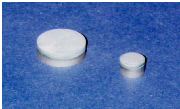
Overall photo of AlN film (full coverage) on tungsten carbide, produced by chemical vapor deposition.
