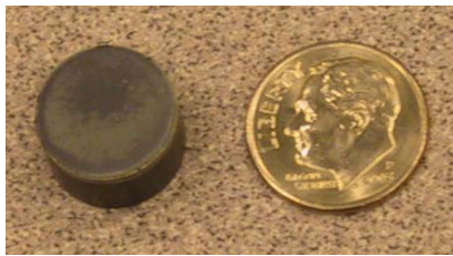
Overall photo of AlN film (full coverage) on SiC, produced by chemical vapor deposition.
