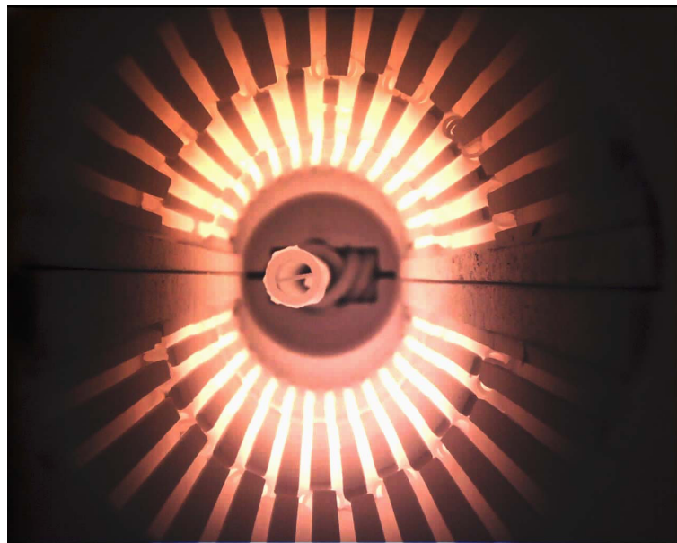
High Temperature Oven Testing of Solids Velocity Probe
