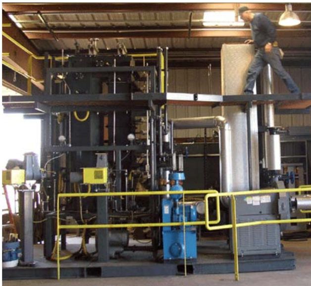
WRI's pilot-scale CTF is ideally suited for flexible testing of coals and combustion processes.
