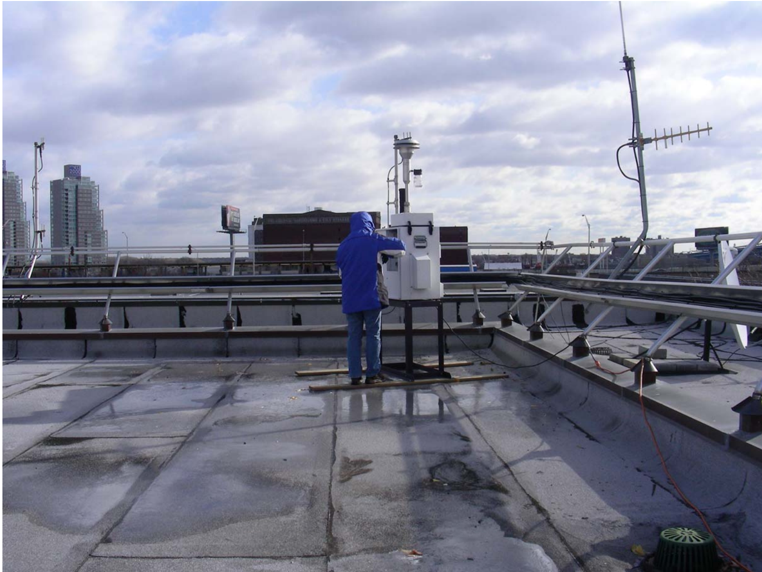
Fire Dept HQ PM 2.5 Sampler on roof.
