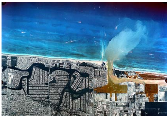
Sediment plume impact on a coastal reef
