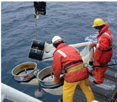
Bongo nets are one of the methods used to collect fishery data
