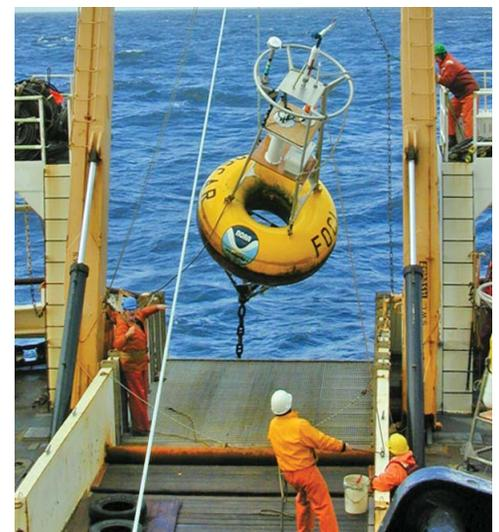
The ship deploys a Fisheries-Oceanography Coordinated Investigations project buoy
