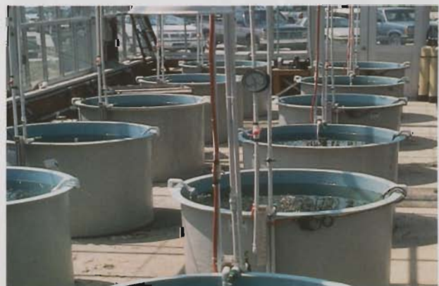
Figure 2-8. Mesocosms set up in a greenhouse at the National Wetlands Research Center. Such mesocosms enable studies of macrophyte responses to discrete variables such as carbon dioxide concentration or salinity.
