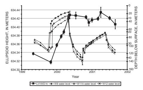
**Figure 7.** Ellipsoid height change of LVVWD GPS station and water-level fluctuations in three adjacent artificial recharge wells. Water-level data were provided by Las Vegas Valley Water District. Error bars on ellipsoid heights are 1-σ.
