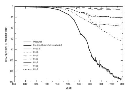
**Figure 5.** Simulated and measured aquifer-system compaction at Franklin, Virginia. (Records correspond to model units in figure 4.)
