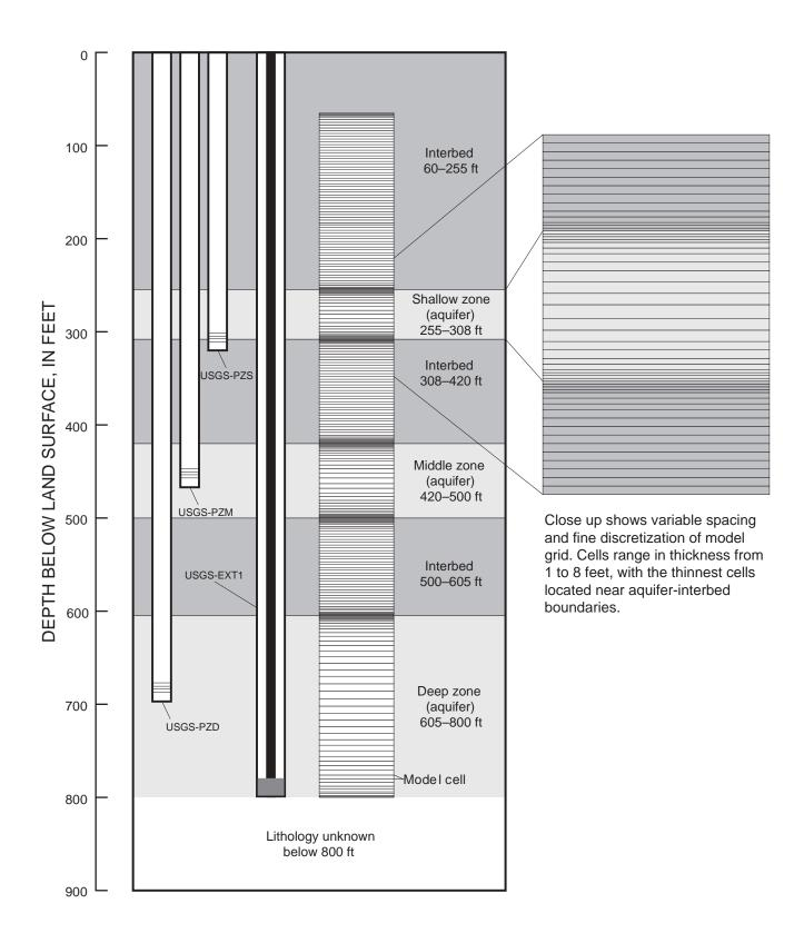
**Figure 2.** Schematic showing piezometer and extensometer depths, aquifer and interbed depths for the Lorenzi model grid, and a close up of the model cells.
