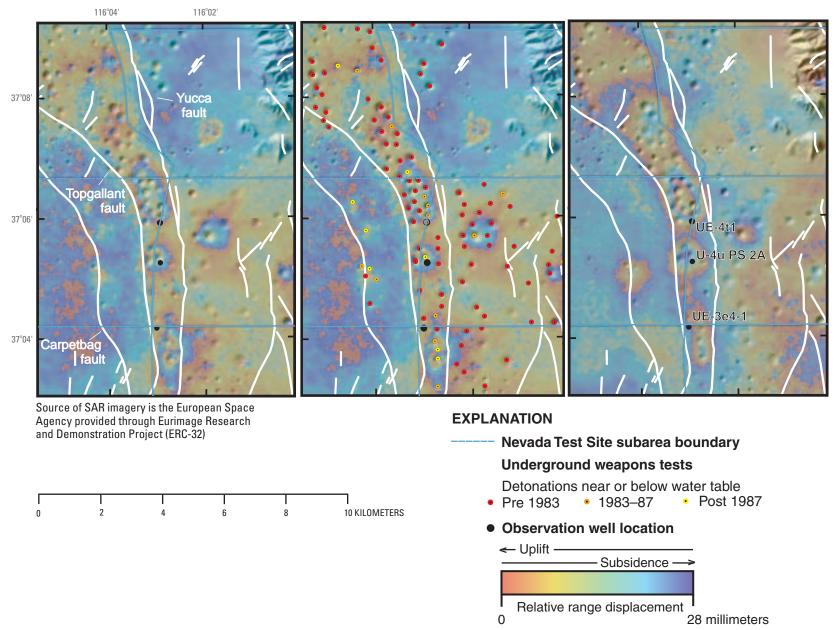
**Figure 3.** InSAR-generated displacement patterns (interferograms) in tuff-pile area of Yucca Flat for three sequential periods spanning 1992–97. First interferogram spans period inclusive of last weapons tests detonated in Yucca Flat area. Middle interferogram shows distribution of tests detonated below water table. Last interferogram identifies long-term observation wells used to measure water-level responses in tuff-pile area.
