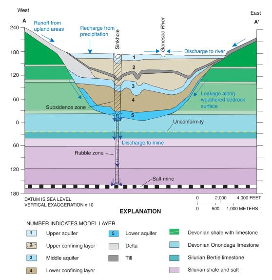
**Figure 2.** Generalized section showing aquifers and confining units in the Genesee Valley (line of section shown in fig. 1).
