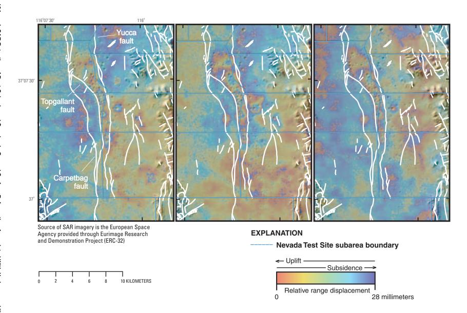
**Figure 2.** InSAR-generated displacement patterns (interferograms) of Yucca Flat area for three sequential periods spanning 1992–97. First interferogram spans period April 24, 1992–June 18, 1993, and is inclusive of the last weapons tests detonated in Yucca Flat area. Remaining two interferograms span sequential periods following the suspension of weapons testing, June 18, 1993–June 11, 1995, and June 11, 1995–June 16, 1997, respectively.
