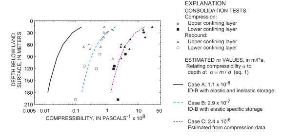
**Figure 3.** Relation of compressibility to depth as derived from consolidation curves of confining-unit sediments in Genesee Valley aquifer system.
