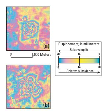
**Figure 4.** Interferograms showing displacement for April 24, 1992–June 18, 1993, caused by two underground weapons tests in Yucca Flat, Nevada. (a) Galena test. (b) Divider test. See figure 3a for locations of the two interferograms.
