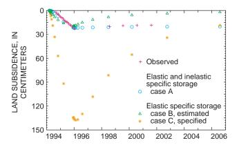
**Figure 7.** Land subsidence measured at monument K10 and predicted by model 1D–B in three alternative regressions.
