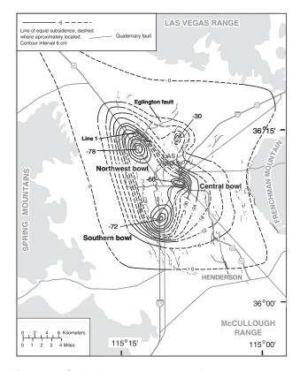
**Figure 2.** Subsidence contour map for 1963–80 showing maximum subsidence in three principal localized bowls in Las Vegas Valley (from Bell, 1981b).
