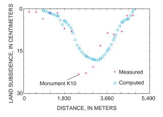
**Figure 8.** Land subsidence along survey line K as measured in February 1996 and as computed by three-dimensional model.
