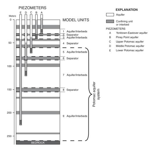
**Figure 4.** Model units for one-dimensional simulation of compaction at Franklin, Virginia. (Piezometers correspond with records of hydraulic head presented in figure 2.)
