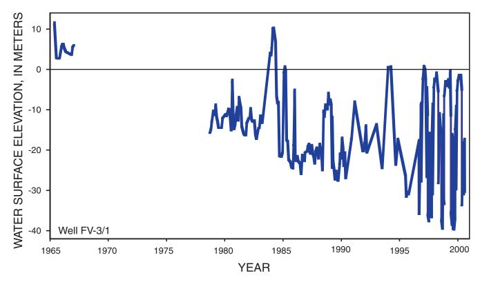
**Figure 5.** Historic water-level fluctuations for well FV-3/1, Santa Ana Basin. Other wells in the region show similar trends. Well is near well X shown in figure 2b.
