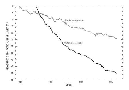
**Figure 3.** Aquifer-system compaction measured by borehole extensometers at Franklin (1979–95) and Suffolk (1982–95).
