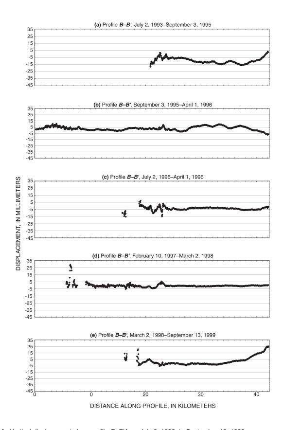
**Figure 4.** Vertical displacement along profile *B–B*' from July 2, 1993, to September 13, 1999.
