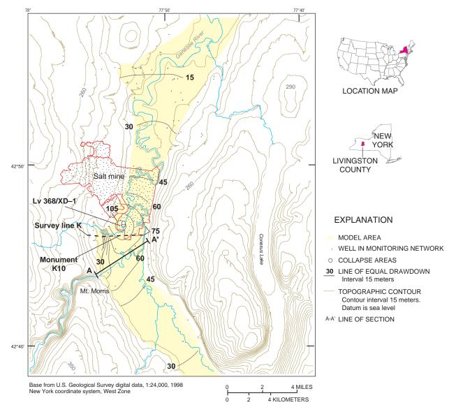
**Figure 1.** Extent of mined area, site of collapse, and distribution of drawdown in lower aquifer in January 1996 in response to mine flooding.
