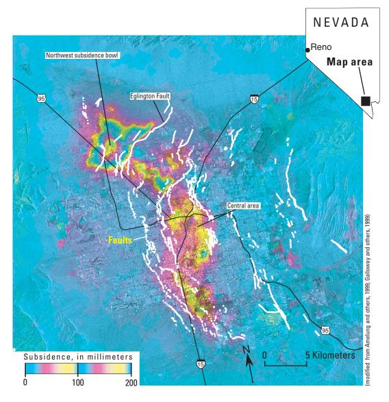
Figure 2. Interferogram showing subsidence for April 21, 1992–December 5, 1997, in Las Vegas Valley, Nevada.
