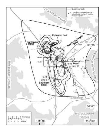
**Figure 5.** Revised subsidence contour map for Las Vegas Valley, 1963–2000, showing maximum subsidence measured in four localized bowls and location of level lines.
