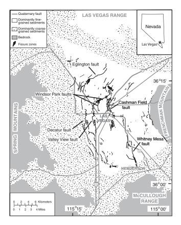
**Figure 1.** Distribution of fine- and coarse-grained deposits and location of principal Quaternary faults, and earth fissures in Las Vegas Valley.
