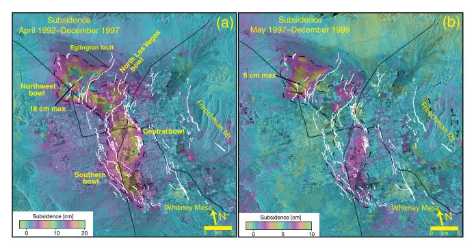
**Figure 4.** Composite interferograms of Las Vegas Valley for (a) April 1992–December 1997 (from Amelung and others, 1999) and (b) May 1997–December 1999. Faults are shown in white.
