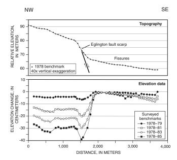
**Figure 3.** Topography and elevation change for level line 1 across the Eglington fault (fig. 2) for the period 1978–85.
