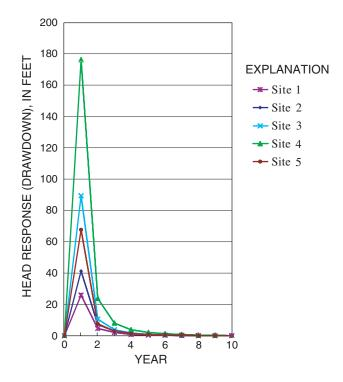
**Figure 5.** Unit response functions at five hypothetical well sites (shown in fig. 3) resulting from 1 year of unit withdrawal (1,500,000 cubic feet per day).
