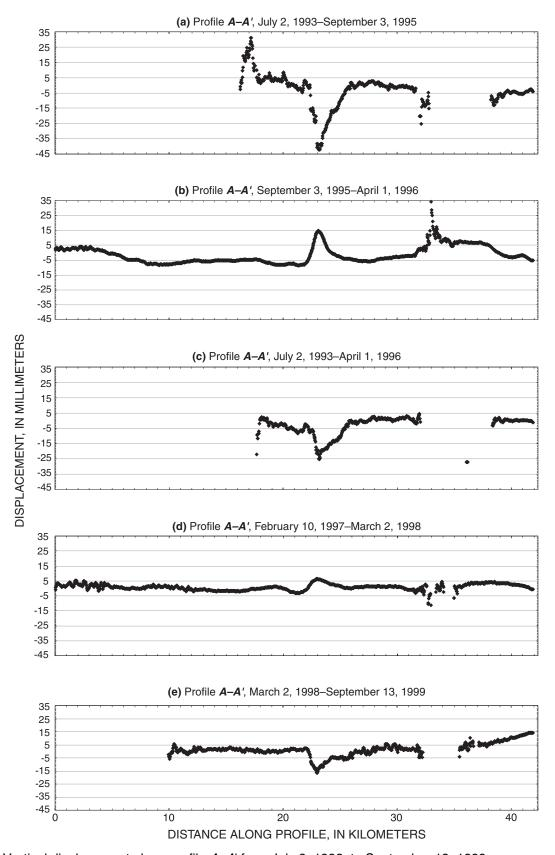
**Figure 3.** Vertical displacement along profile *A–A*<sup>1</sup> from July 2, 1993, to September 13, 1999.
