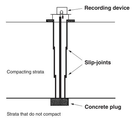
Figure 2. Extensometer used by HGCSD.
