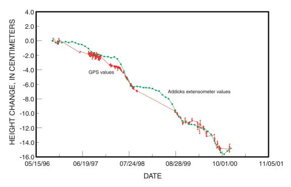
**Figure 13.** Comparison of techniques to estimate subsidence—Addicks extensometer values versus PAM 05 GPS ellipsoid height values.
