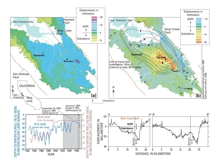
**Figure 1.** Land-surface displacement and hydrographs for wells 7S/1E–16C05 and 6S/2W–24C07 in Santa Clara Valley, California. (a) Interferogram for September 23, 1992–August 2, 1997 (5 years). (b) Subsidence contours for 1934–67 and interferogram and two cross sections for January 4, 1997–August 2, 1997 (8 months).
