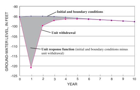
**Figure 4.** Response of the Chicot aquifer at well site 2 to initial and boundary conditions and to a unit withdrawal of 1,500,000 cubic feet per day for 1 year.
