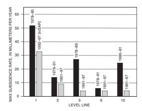
**Figure 6.** Histogram showing maximum subsidence rates measured along level lines 1, 2, 3, 6, and 10 (fig. 5) for the period 1978–97. Pre- and post-1991 rates are compared for each line on the basis of conventional leveling results, except for line 1 which is based on post-1991 InSAR measurements.
