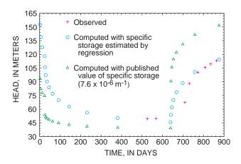
**Figure 4.** Water levels predicted from two alternative values of  $S_s$  and measured in the lower aquifer at well Lv368 near the collapse area.
