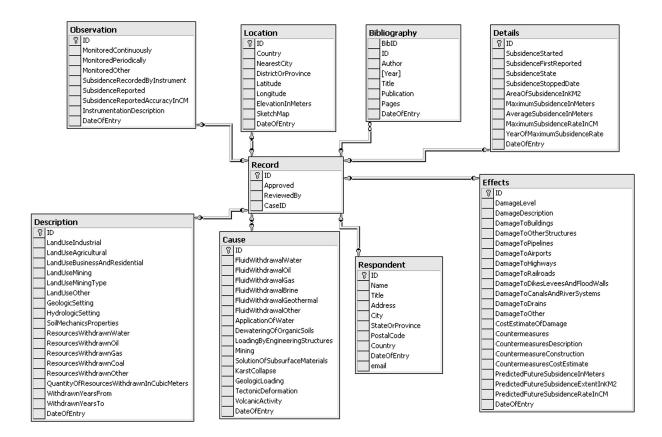
Figure 1. Diagram showing data base functional relations.
