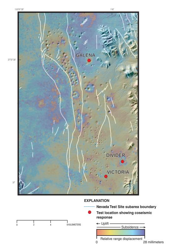
**Figure 5.** Location of three weapons tests detonated in 1992. All three tests were detonated above the water table. Interferogram spans period of tests April 24, 1992–June 18, 1993
