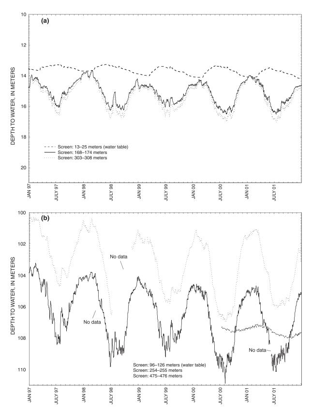
**Figure 5.** Depth to water in (a) Garfield piezometers and (b) Del Sol Divider piezometers. (Location of piezometer sites in figure 2d.)
