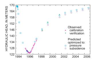
**Figure 5.** Hydraulic head in upper confining unit near collapse area as computed by one-dimensional model 1D–A and measured at borehole XD–1.
