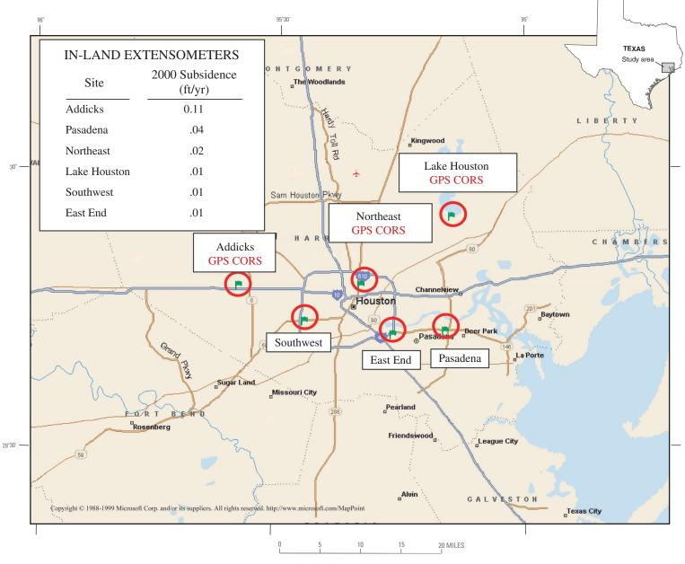
**Figure 4.** Locations of the three GPS CORS colocated with borehole extensometers, locations of other project borehole extensometers, and rates of subsidence in six extensometers in the Houston-Galveston region, Texas.
