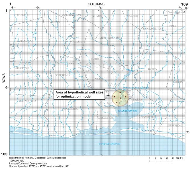
**Figure 2.** Ground-water-flow model grid and location of hypothetical well sites used in the optimization model of the Houston area, Texas.
