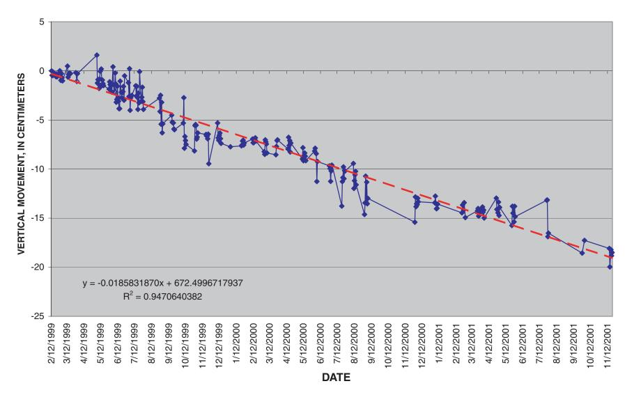
Figure 11. Ellipsoid height differences between Lake Houston CORS and PAM 07 site.
