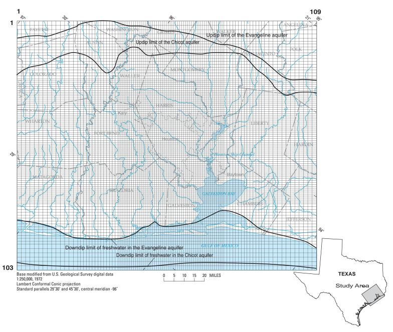
Figure 1. Location of study area with finite-difference grid used in the numerical model of the Chicot and Evangeline aquifer system.
