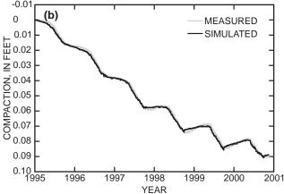
**Figure 3.** Estimated, measured, and simulated compaction at the Lorenzi site for (a) the historical period, 1901–94, and (b) the recent period, 1995–2000.
