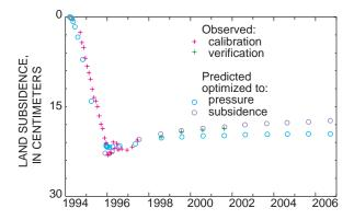
**Figure 6.** Subsidence computed by one-dimensional model 1D–B and measured land subsidence at monument K10, 850 m south of collapse area.
