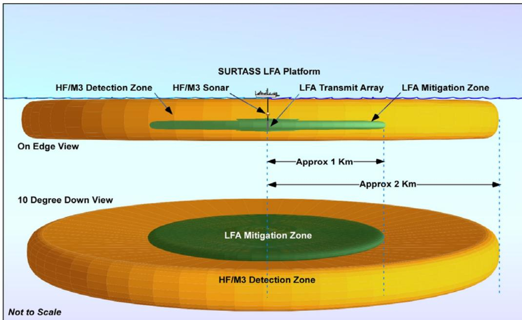
Figure 2. HF/M3 Sonar Detection and LFA Mitigation Zones
