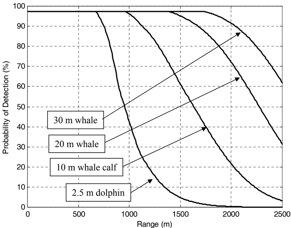
Figure 5. Probability of Detecting (on any given ping) Various Marine Mammals Swimming within the Search Beam of the HF/M3 Sonar System
