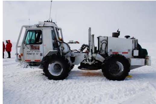
Figure 3: 20,000 lb mini-vibrator (to be modified for tracks).
