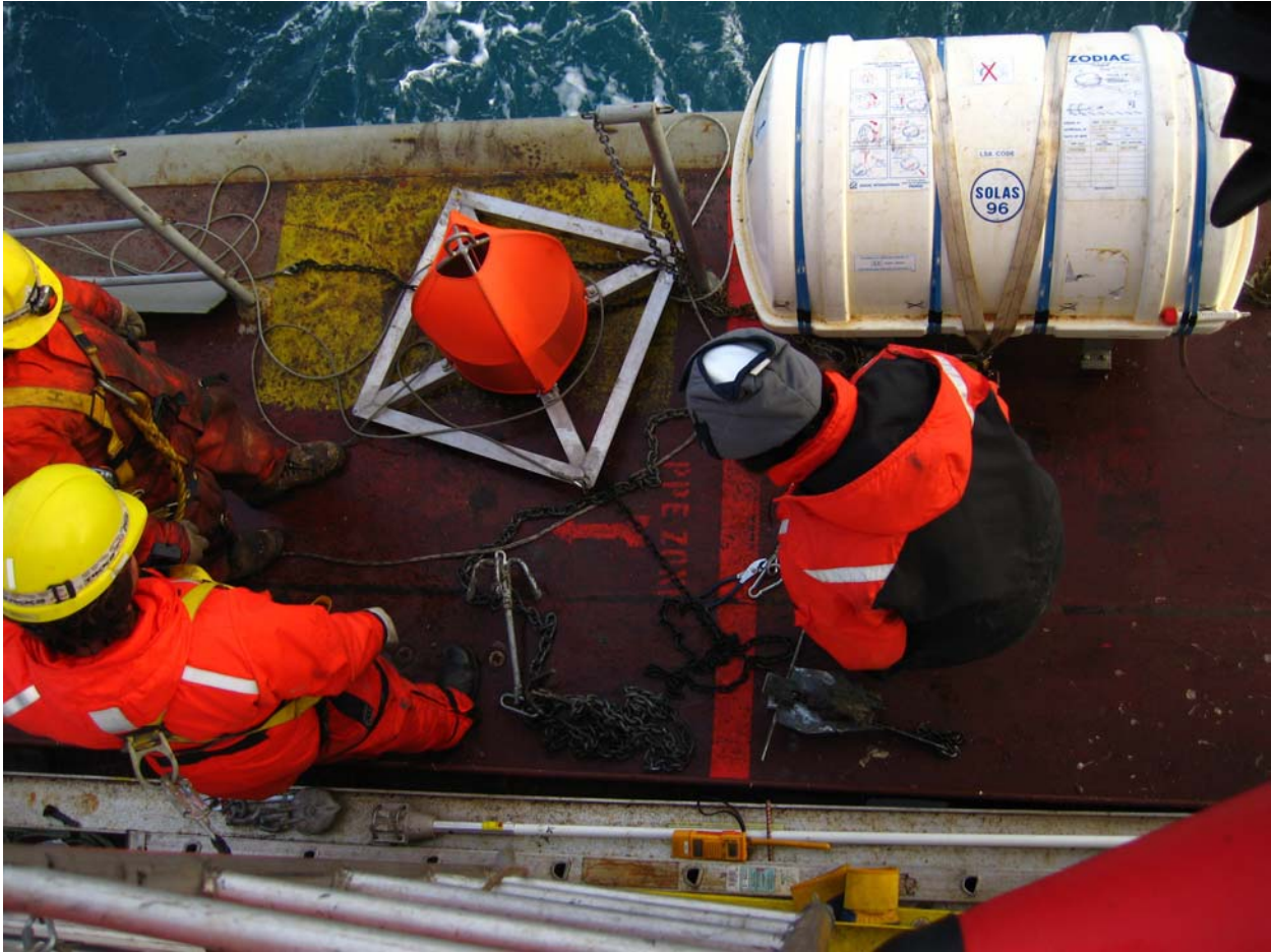
FIGURE 10.2. Photograph of a DASARb on deck after retrieval. Note the latex sock over the frame and a grapnel anchor and chain on the deck.
