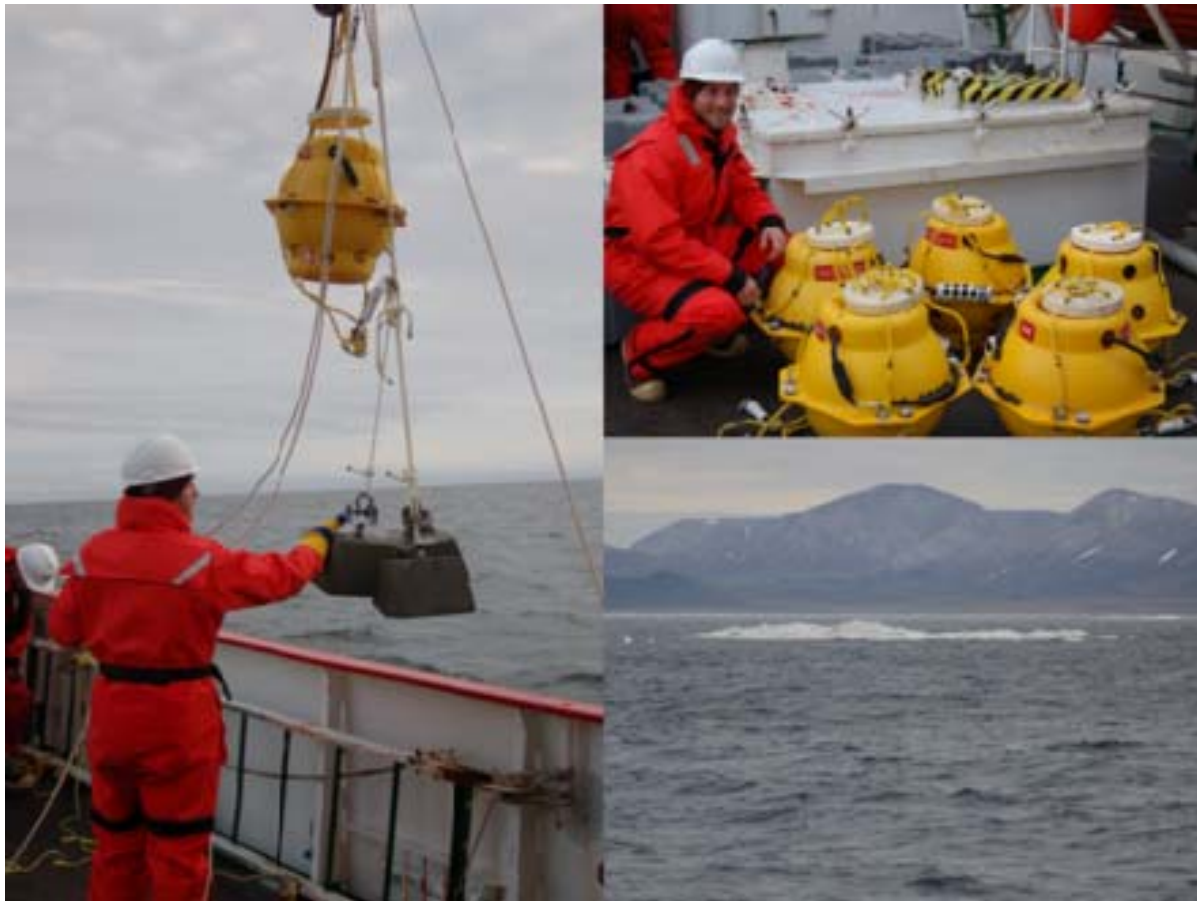
Figure 6.1 Autonomous seafloor recorders, referred to as “pop-ups” during deployment off Cape Lisburne, Alaska.
