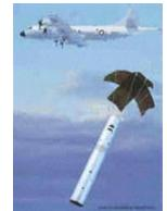
Figure C-12. MPA deploying AN/SSQ-110A
