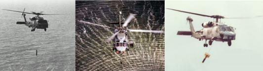
Figure C-10. AN/AQS-22 being deployed by SH-60 helicopter
