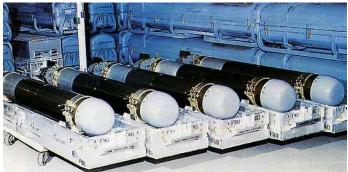
Figure C-24. MK 54 Torpedoes
