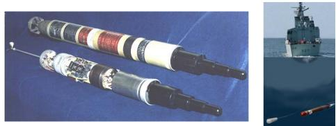
Figure C-25. ADC CM (L), and AN/SLQ-25 (NIXIE) CM (R)
