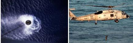
Figure C-9. AN/AQS-13 being deployed by SH-60 helicopter
