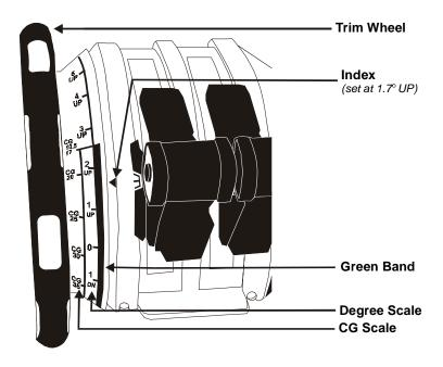
Figure 1. Airbus THS Trim Wheel Indicator Scales.
