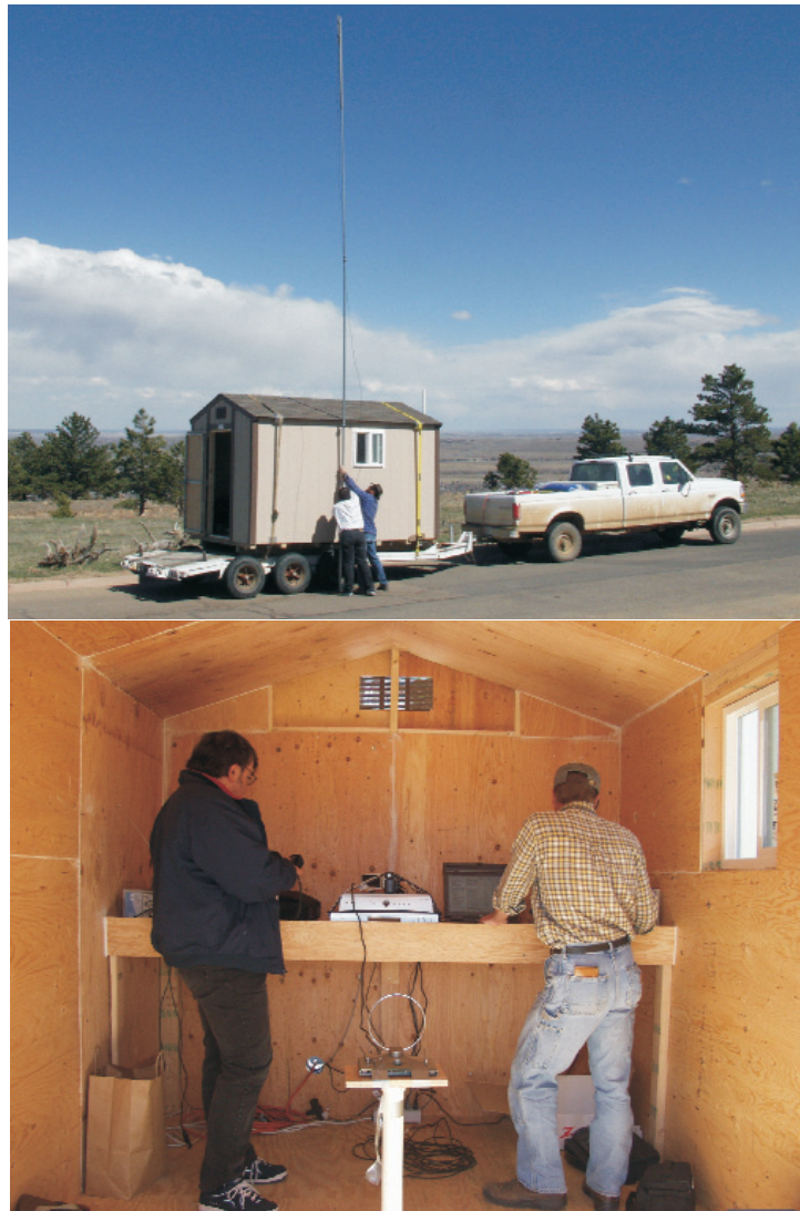
Figure 1. Outside (top) and inside (bottom) of the ITS “Tool Shed Measurement System,” used in the DTV field strength and video quality study (photographs by W.A. Kissick).
