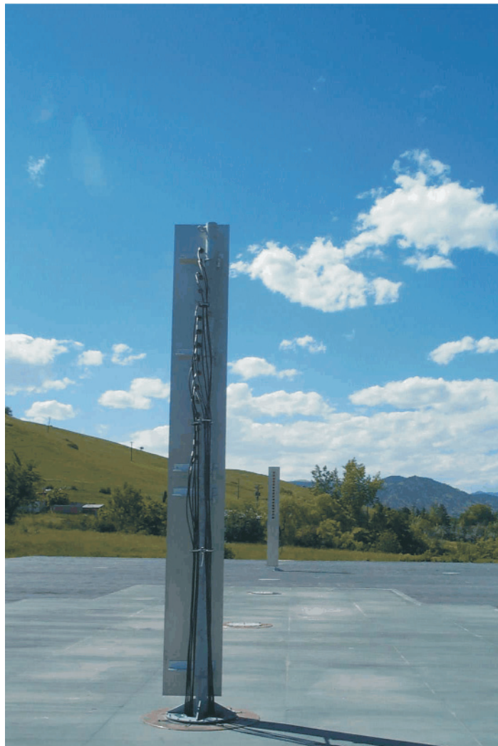
Figure 1. 16-element transmit and receive antenna arrays used for MIMO testing at the NIST open area test site. The closer array is the receiving antenna (photograph by P. Papazian).
