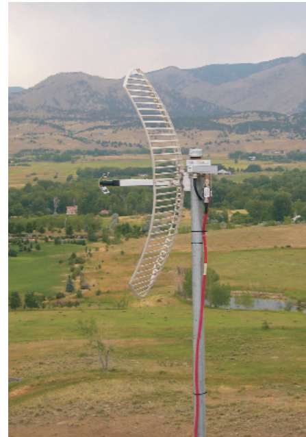
Figure 3. High gain directional antenna employed at one outdoor link at the Table Mountain field site (photograph by C. Redding).
