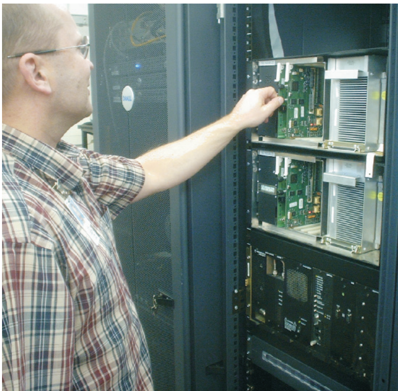
Figure 2. An ITS engineer making equipment configuration changes on land mobile radio base station equipment in the ITS Interoperability Research Laboratory (photograph by E. Gray).
