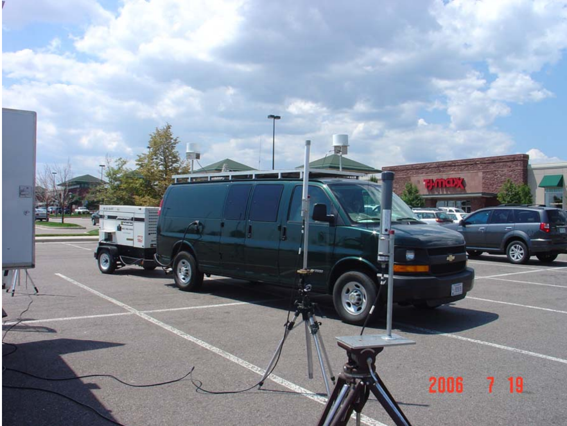
Figure 3. The 5.8 GHz and 2260 MHz transmitter antennas that were used in mall parking lot measurements.
