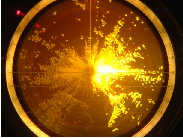
Figure 1. An example of clutter on a 9-GHz maritime radionavigation radar display. The clutter includes local buildings, terrain, and vegetation. No intentional interference or test targets are present on this display.
