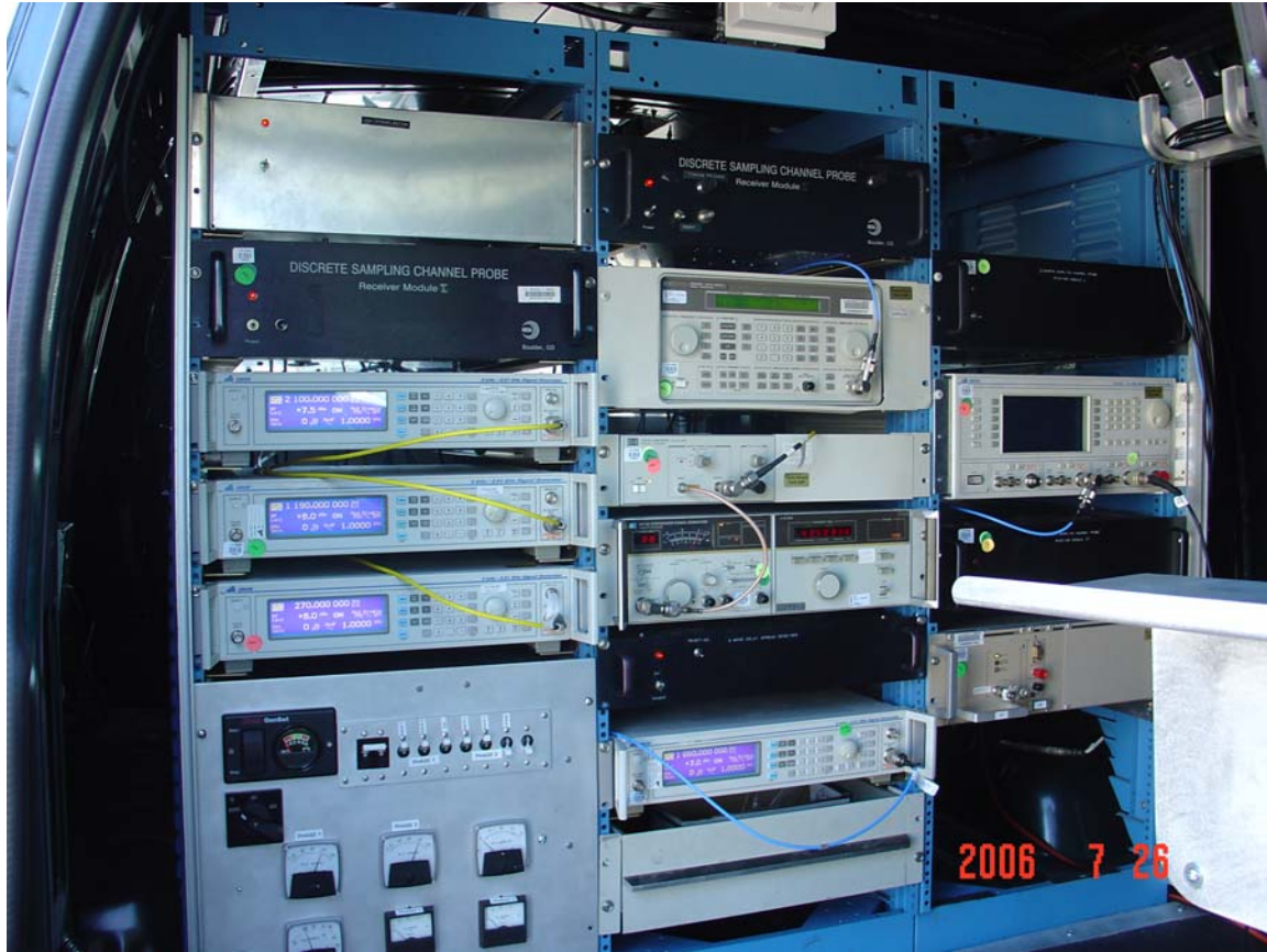
Figure 2. The measurement van configured with an 8 channel receiver.
