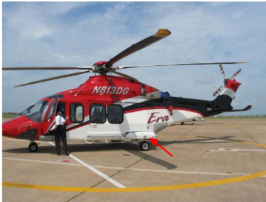
Figure 2. An external liferaft pod on an Agusta Westland AB139 helicopter (as indicated by the red arrow).
