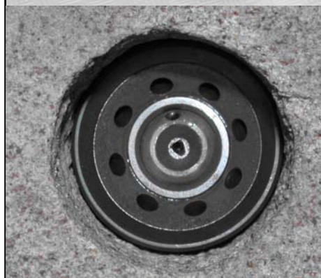
Tempress jet drill (top). Sandstone showing, 1.165-inch diameter tool face and tight-gage hole (bottom).
