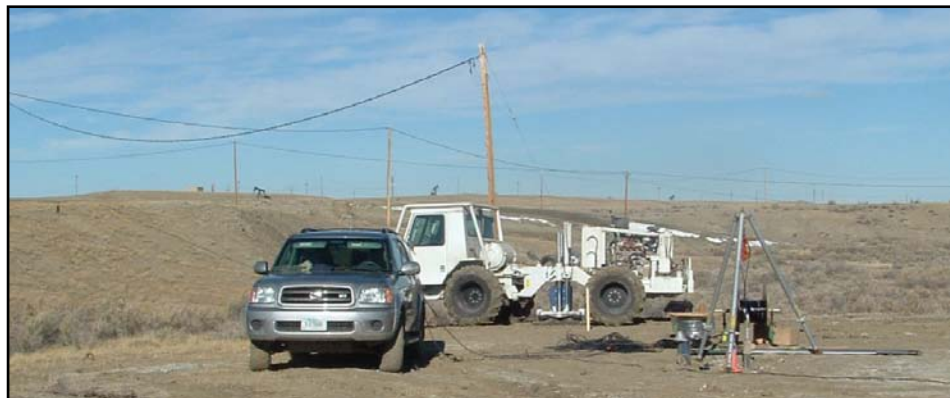
The complete system used to acquire the VSP data. The simplicity of the system allowed for hand deployment, a rental vehicle for the “doghouse,” and a small vibrator for the source. Note the small tripod used to support the sensor string; normally, a workover rig and many more personnel are needed.
